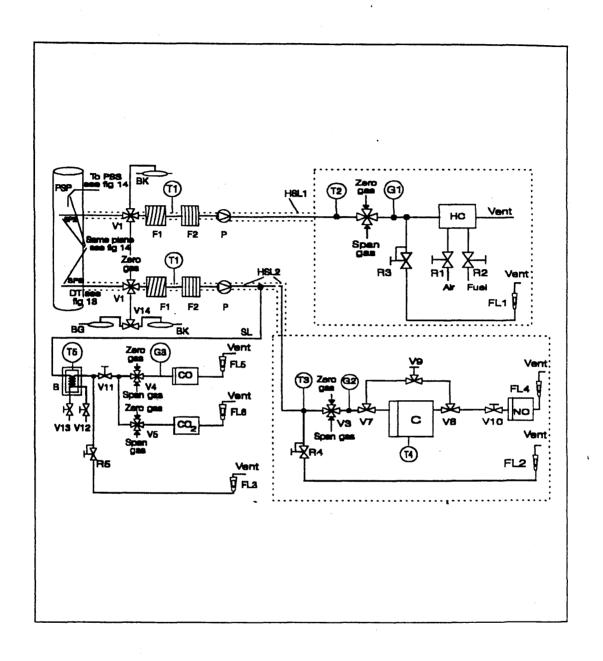
Figure 3 Flow Diagram of Dilute Exhaust Gas Analysis System for CO,  $\mathrm{CO_2}$ ,  $\mathrm{NO_x}$  and HC
