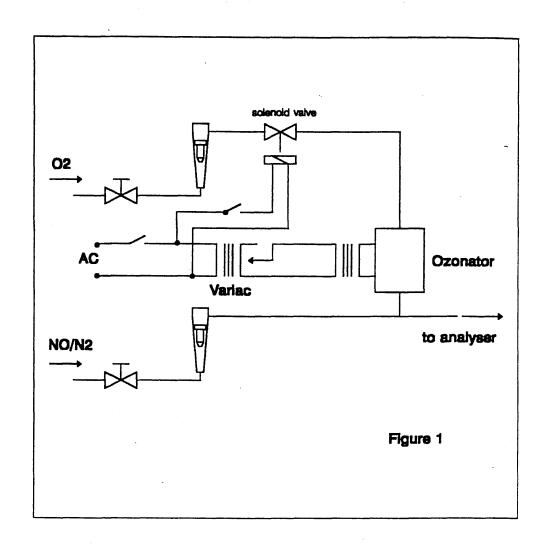
Figure 1 Schematic of NO<sub>2</sub> converter efficiency device
