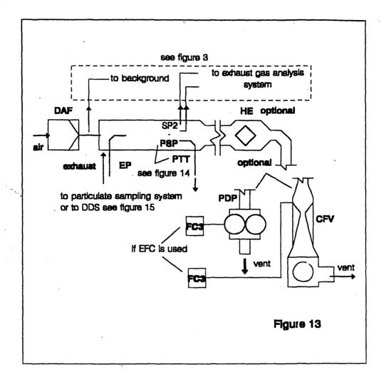
The total amount of raw exhaust gas is mixed in the dilution tunnel DT with the dilution air.
