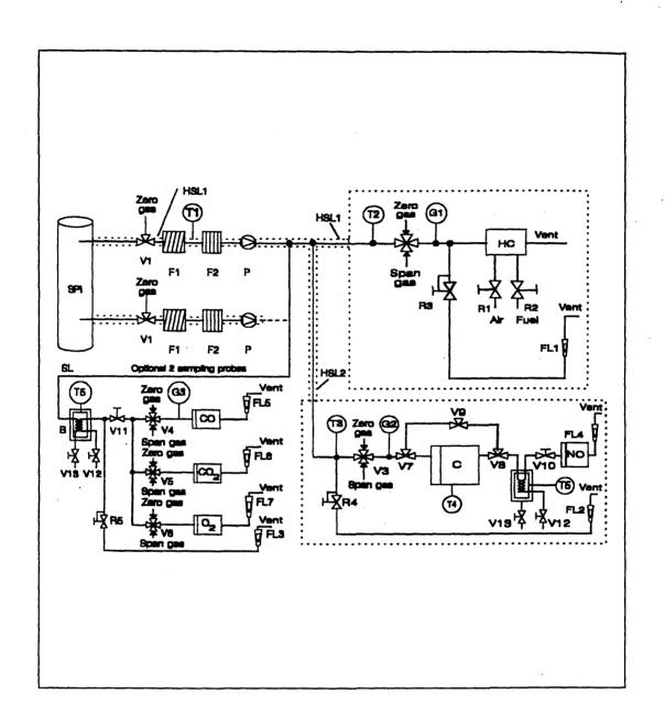
Figure 2 Flow Diagram of Exhaust Gas Analysis System for CO,  $\mathrm{NO}_{\mathrm{x}}$  and HC
