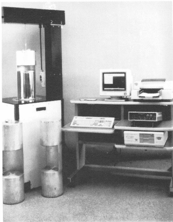
Fig. 2. Photograph of the Passive/Active NCC system.
