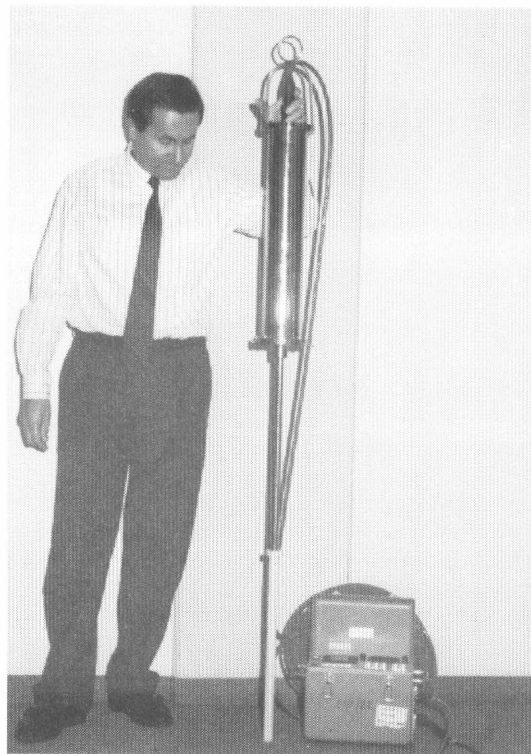
Figure 3 - OVERALL VIEW OF A SPENT FUEL ATTRIBUTE TESTER FOR FUEL WITH LONG COOLING TIME
