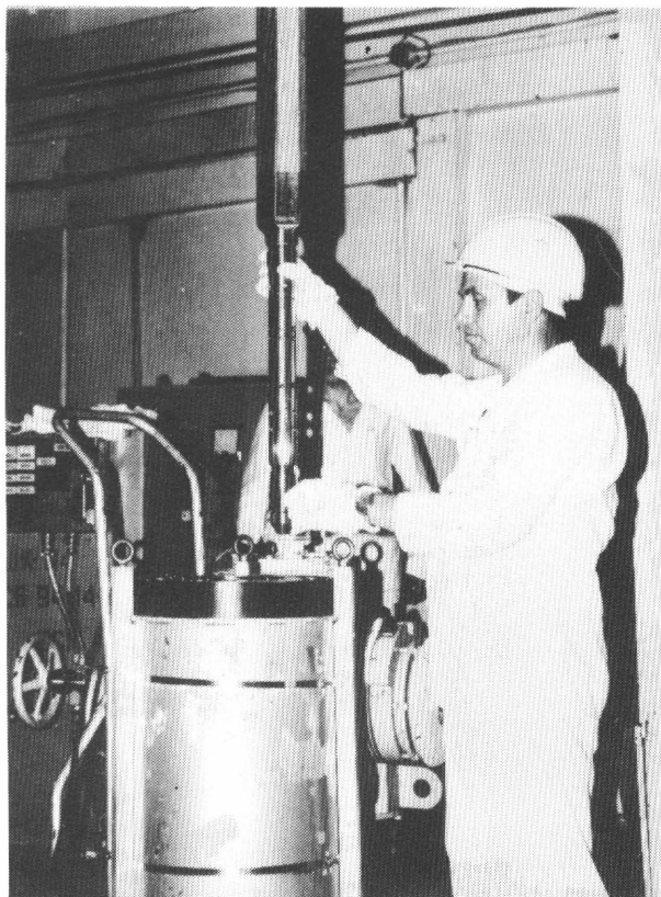
Fig. 4. BN600 fuel assembly being positioned for lowering into the AWCC.
