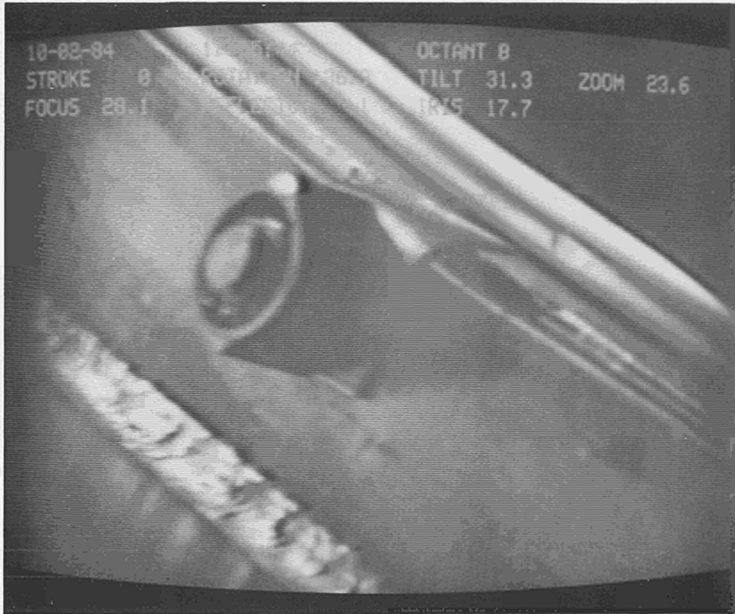
Fig. 71 View of protection plate rail taken with in-vessel inspection camera.
