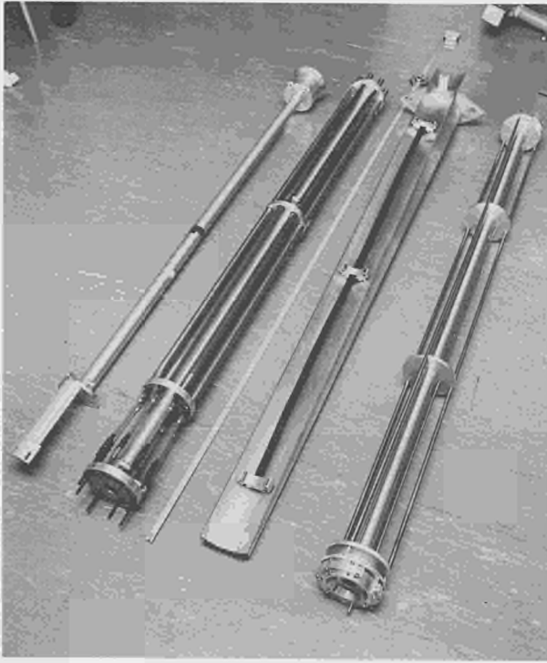
Fig. 65 Set of tools for handling RF transmission line components.
