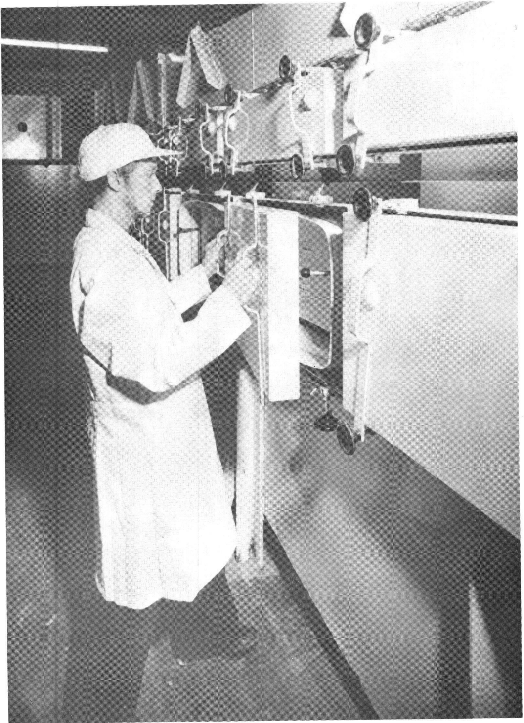
Fig.6 Photo: Unipak Housing showing cam operating handles and location domes in closure doors.
