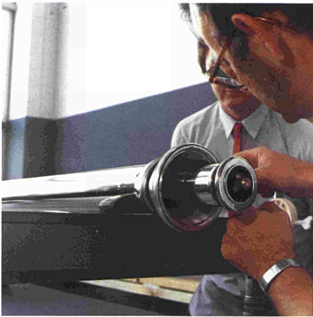
Fig. 43 A vacuum transmission line and interface for the A_1 antenna. A net forward power of 1.5 MW is transmitted through this reduced section. 85.T.1298c/4
