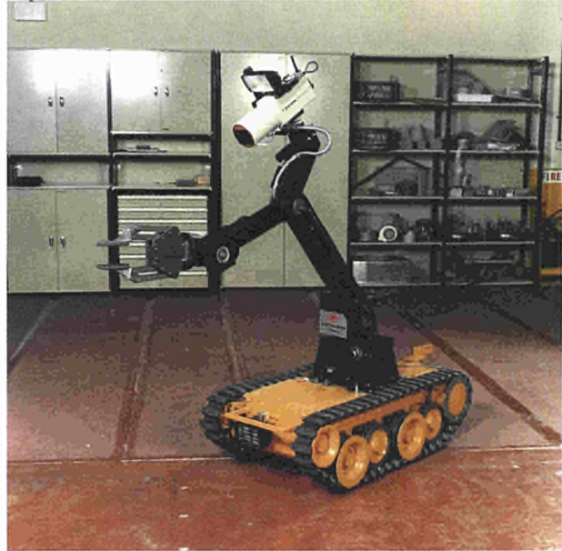
Fig.47 The battery operated roving vehicle for carrying a simple manipulator and TV cameras. 86.T.118c/4
