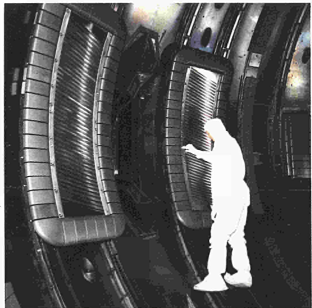
Fig. 42 Two of the three prototype A_0 antennae installed in the vacuum vessel. These antennae were coupling 6 MW of power to the plasma by the end of 1985 and are expected to be used throughout 1986.
