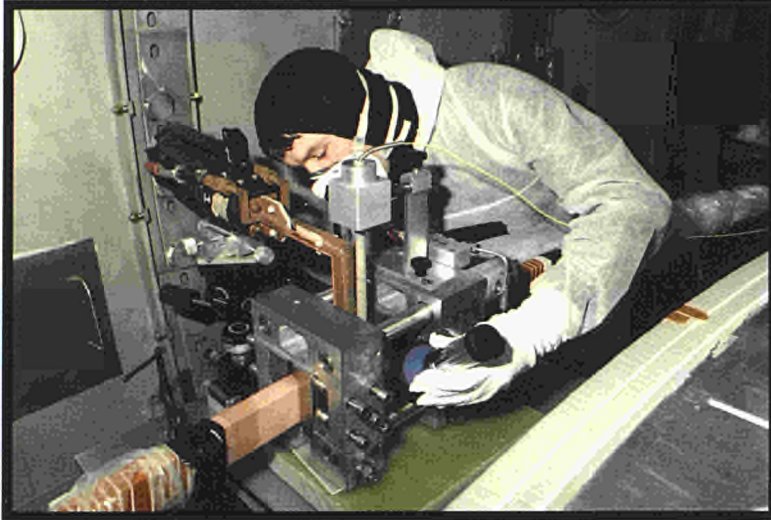
Fig. 7: Brazing jig and brazing coil mounted on a joint
