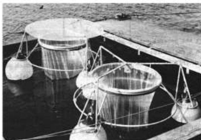
Fig. 1: Plastic enclosures (contents 1.5 m 3 ) anchored in the harbour of Den Helder, the Netherlands.
