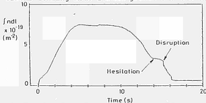
Fig 5: Time dependence of electron line density showing hesitation before disruption.
