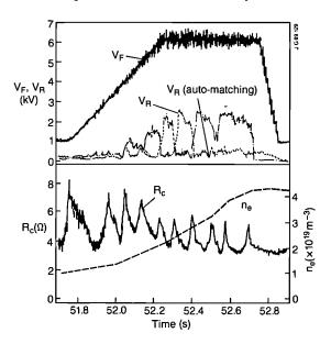
Fig.27: Typical evolution of signals during high power ICRF heating.  $V_{\rm F}$ ,  $V_{\rm R}$ ,  $R_{\rm C}$ : forward and reflected voltages and loading resistance of one half antenna.  $n_{\rm e}$ : plasma electron density. Total power 10MW. The auto-matching network provides a low reflection coefficient despite large variations in the load resistance and reactance.
