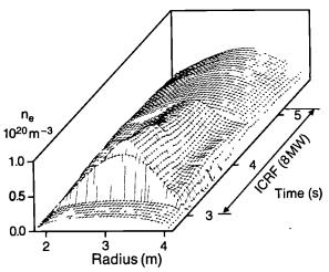
Fig. 65 Electron density profile after pellet injection and reheat by ICRF. Note the peaked  $n_e$  profile which relaxes at the same time as  $T_e(R)$ .
