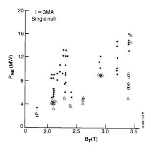
Fig.78: H-Mode threshold power as function of toroidal magnetic field (I=3MA, single null X-point).
