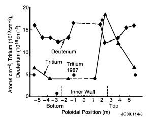
Fig.119: The poloidal distribution of tritium in the walls of JET measured after the 1986 and 1987 campaigns. Analyses of the tritium was carried out using liquid scintillation counters.
