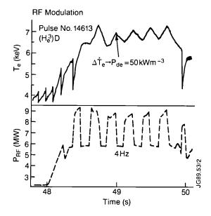
Fig.135: Response of the electron temperature to 4Hz modulation of the ICRF power. The discontinuity in (dT<sub>e</sub>/dt) corresponds to a modulated direct heating power density of 50kW/m<sup>3</sup>.
