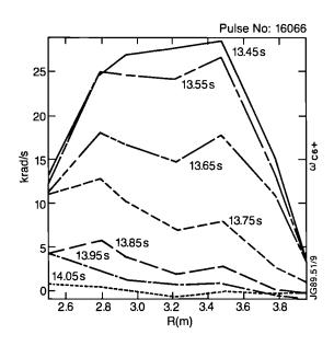
Fig.132: The ion toroidal rotation profiles across the plasma radius during the drop in the rotation frequency at mode locking.
