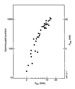
Fig.49: Variation of count-rate of 16.5 MeV gamma rays (l.h.s) and related fusion power (r.h.s) from D(<sup>3</sup>He,p)<sup>4</sup>He reactions with applied rf power tuned to minority <sup>3</sup>He ions.
