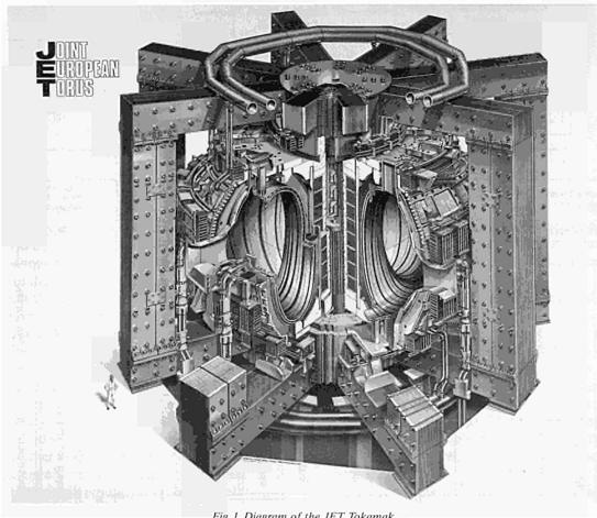
Fig. 1 Diagram of the JET Tokamak
