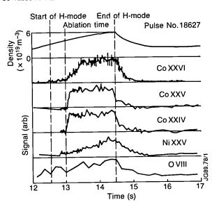
Fig.52 The time development of the line average electron density and the emission from cobalt, nickel and oxygen lines following the injection of some cobalt by the laser blow-off system. The injection takes place during an H-mode.
