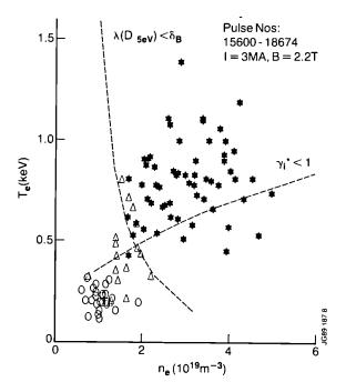
Fig.81: Edge temperature  $T_e(\chi=0.95)$  versus edge density  $n_e(\chi=0.95)$  for OH(0), L-( $\Delta$ ) and H-mode (\*) discharges (I=3 MA, B=2.2 T).
