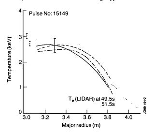
Fig.48: Showing ion and electron temperature profiles for a typical 5MA discharge. The electron temperature profiles are from ECE (thin, dotted line) and Lidar (thin, dashed lines) diagnostics. The ion temperature profiles (heavy lines) and derived from the Neutron Profile Monitor using three different analytical procedures. The error bar shows the typical absolute accuracy.
