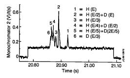
Fig.26: Doppler-shift spectrum using differing gases for source and neutraliser.
