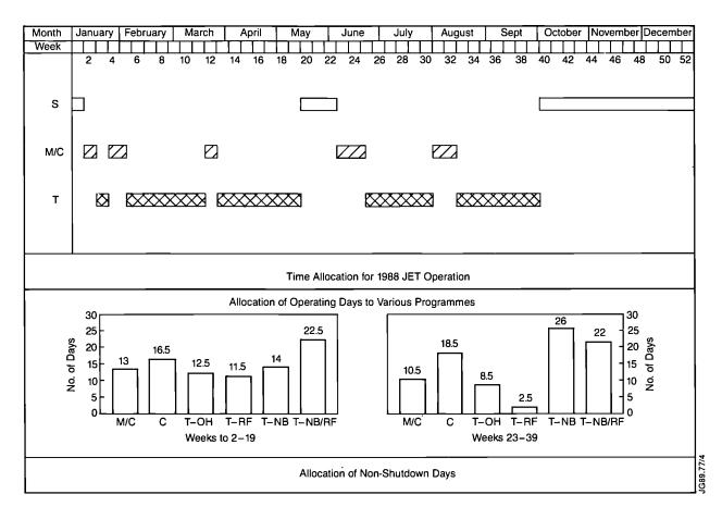
Fig 58: Allocation of time to different activities of the operating programme for 1988 (S=Shutdown; M/C=Machine Commissioning; T=Tokamak Operations).
