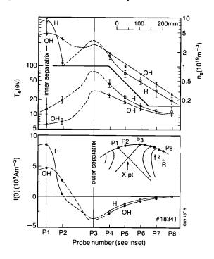
Fig.82: Profiles of density, temperature and ion saturation current in front of the target plates, measured with Langmuir probes mounted in these plates.
