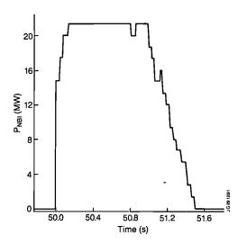
Fig.17: Injected power waveform for Pulse No:18569; 16 beam sources operating at 80kV in deuterium.
