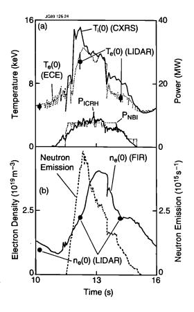
Fig.94: Data for JET Pulse No.16066, (a) central temperatures and additional heating powers versus time, (b) the central electron density and neutron emission rate versus time.
