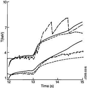
Fig.102: Results of the simulation of an H-mode discharge at 4MA (Pulse No:16297): a) time evolution of energy content from models (PT—, RL ...) and measurements (magnetic ---, diamagnetic ---); b) time evolution of central and average Te from models (PT—,RL ...) and ECE (---)
