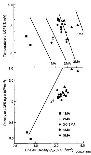
Fig.107: Scaling of T<sub>e</sub> and n<sub>e</sub> at the LCFS with line average density, T<sub>e</sub>.
