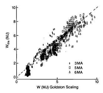
Fig. 67 Comparison of 3, 5 and 6MA data with the Goldston (Aachen) scaling. 3MA performs better and 6MA is worse.
