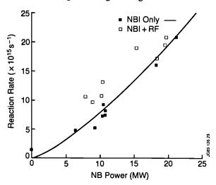
Fig.99: Reaction rate versus neutral beam power, solid points NBI only, open points with the addition of ICRH.
