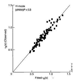
Fig.85: Observed versus fitted energy confinement times from an ordinary least squares fit.
