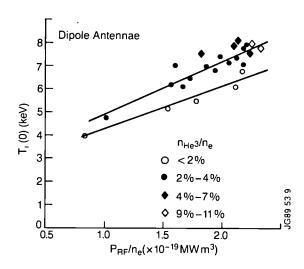
Fig.134: Central ion temperature versus  $P_{RF}/n_e$  for various <sup>3</sup>He minority ion concentrations.
