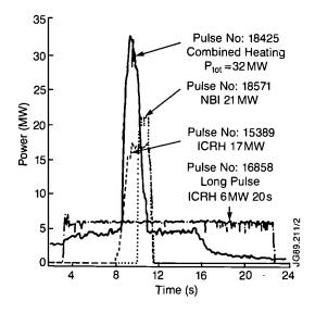
Fig.145: Power delivered to JET plasmas as a function of time. In particular, combined heating power (NB+RF) has exceeded 32MW in the plasma.
