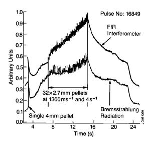
Fig.89: Bremsstrahlung and FIR-interferometer signal for demonstration of fuelling experiments: Pulse No. 16849, 4mm pellet at 3s and 32 2.7mm pellets at 4s<sup>-1</sup> starting at 7s into the plasma pulse.
