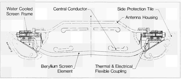
Fig.29: Cross-section of the ICRF antenna equipped with the new beryllium screen.
