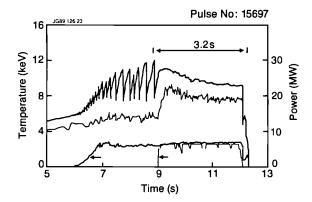
Fig.93: Behaviour of the central electron and ion temperatures during the longest period of sawtooth stabilization observed.
