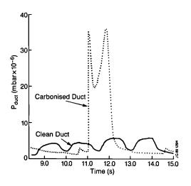
Fig.20: Typical duct pressure traces for 1s, 2 beam pulses during duct conditioning sequence. In each case the duct had been exposed to a few beam seconds of conditioning.
