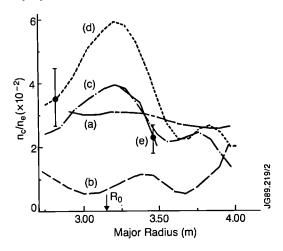
Fig.104: Sequence of radial profiles of carbon concentration, using the VB measurement, for a pellet injection fuelled plasma. (a) is the pre-pellet equilibrium profile, (b), (c) and (d) are respectively at 0.1 s, 0.9s and 1.2s after pellet injection. Profile (e) is from the CXRS measurements, and corresponds to (c) temporally.
