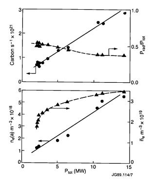
Fig.114: The ICRH power scaling of the carbon influx from the lower belt limiter, the radiated power fraction  $P_{rad}/P_{tov}$ , the edge density  $n_e$  (a) and the volume-averaged density  $\overline{n}_e$  in a 3.3 MA discharge.
