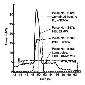
Fig. 62 Power traces corresponding to highest performance of the heating systems either used alone or combined.
