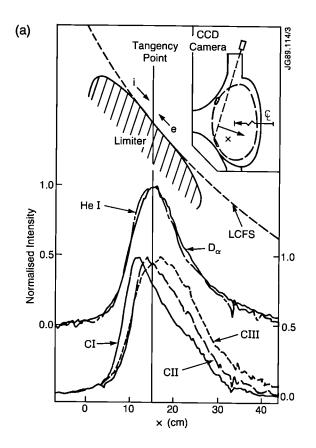
Fig.113(a): Spatial distributions of the low ionisation states of C I, C II, C III, He and  $D_{\alpha}$  around the lower belt limiter in a 3.1 MA discharge with  $\bar{n}_{\tau} = 1.5 \times 10^{19} m^{-3}$
