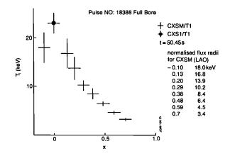
Fig.95: Ion temperature profile charge exchange recombination spectroscopic measurements for a high power (20MW) neutral beam heated discharge.
