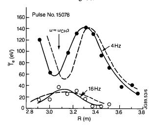
Fig.136: Radial profiles of the modulated temperature in response to 4 Hz and 16 Hz RF power modulation. Note the central minimum  $(R \approx 3.1 \text{m})$  for the 4 Hz case.
