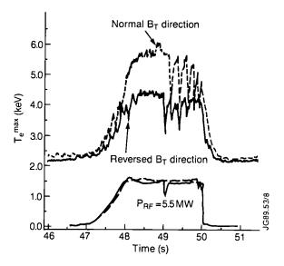
Fig.133: Time evolution of central electron temperature during ICRH with normal and reversed toroidal field directions.
