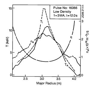
Fig.146: Radial profiles of electron and ion temperatures, electron density and safety factor in a 3 MA, low density discharge with  $B=3.1\,T$ ,  $P_{RF}=8MW,\,P_{TOT}=16.5\,MW,\,Z_{eff}=5.2,\,T_E=0.4\,s.$
