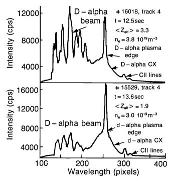
Fig.57 Balmer Alpha spectra of plasma edge, thermal deuterons and fast injected neutrals for two JET pulses with comparable densities but different effective ion charge  $Z_{\rm eff}$ .
