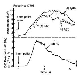
Fig.88: (a)  $T_e$  (0) from ECE; (b)  $T_i$  (0) from the Crystal Spectrometer; (c)  $T_i$  (0) from the Charge-Exchange Spectroscopy; and (d) total neutron rate versus time (4 mm pellet event at 3 s into the pulse) for Pulse No. 17706.
