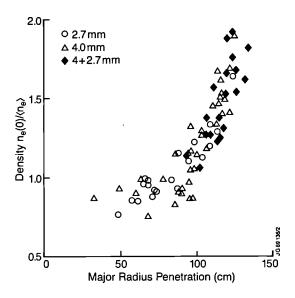
Fig.87: Ratio of density peaking factors,  $\alpha = n_e(0)/< n_e>$ , before and 0.2s after the pellet event;  $\alpha$  after the event in absolute value has to be multiplied by about 1.5.
