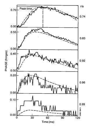
Fig.45: Comparison of model predictions (dotted curves) with measurements (solid curves) for five different reflectometer channels. The best fit is obtained with the particle diffusion coefficient  $D_p(r) = (0.16 \pm 0.02)(1 + 2r^2/a^2) \, m^2 s^{-1}$  for r/a in the range 0.58 < r/a < 1.0.
