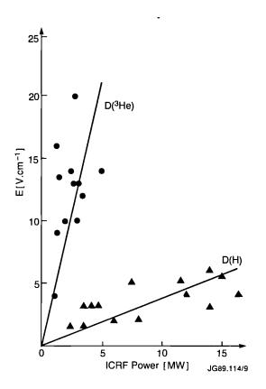
Fig.109: Electric field strength in the scrape-off layer during ICRH for the different minority species  $^3$ He and H ( $I_p$  = 3 MA,  $B_T$  = 3.4 T)
