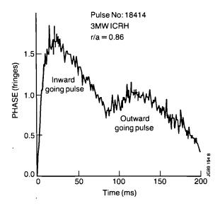
Fig.44: Response of the reflectometer channel probing the layer at r/a=0.86 following a sawtooth collapse. The inward and outward going density pulses are clearly seen.
