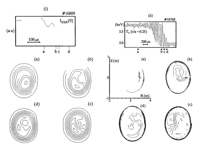
Fig.123: Comparison of sawtooth collapses in JET using (i) SXR and (ii) ECE reconstruction techniques. In both cases a characteristic displacement of the plasma core and formation of a crescent-shaped hot region can be observed. This is followed by a rapid cooling of the displaced core. Successor oscillations are due to the rotation of the plasma residue of the crescent-shaped region.
