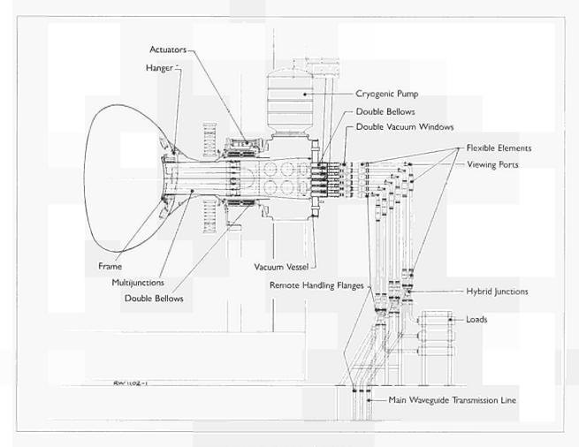
Fig.151: Schematic diagram of LHCD launcher;
