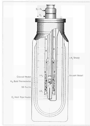
Fig.154: Cryotransfer Pump
