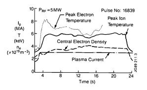
Fig.144: Quasi-stationary plasma exceeding 30s in duration at temperatures in excess of 5 keV. The 3 MA plasma was heated by 5 MW ICRF power.
