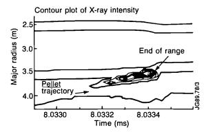
Fig.50 Contour and 3-D plots of the pellet ablation, as seen by the vertical camera. X-ray intensity is plotted versus time and major radius. The peak at the inner edge is an  $H_{\alpha}$  ghost and should be ignored.
