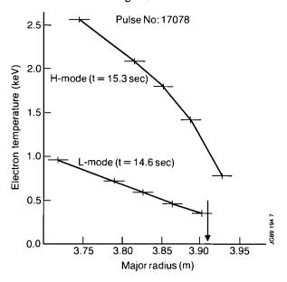
Fig.42: Edge electron temperature profiles measured by the heterodyne radiometer on a plasma exhibiting an L-mode to H-mode transition. The horizontal bars indicate the calculated spatial resolution. The arrow shows the position of the magnetic separatrix calculated from magnetic measurements.
