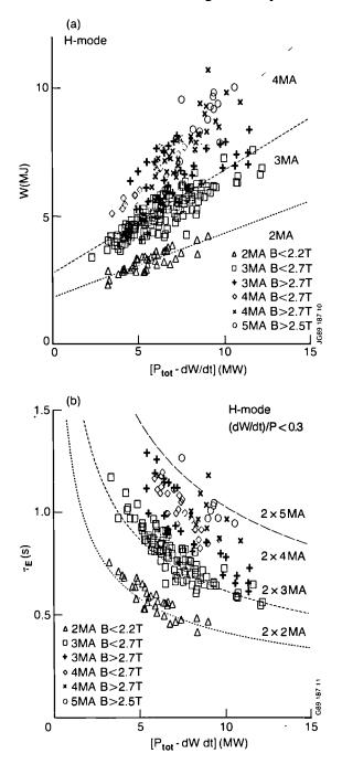
Fig.83: (a) Plasma energy and (b) global energy confinement time in ELM-free H-mode plasma versus total net input power for currents of 2, 3, 4 and 5 MA.
