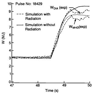
Fig. 69 Simulation of 25MW, 6.2MA heating pulse by a local transport code using the Rebut-Lallia transport coefficients. The code uses the measured electron density and radiated power and self-consistent power deposition profiles.
