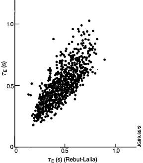
Fig.100: Observed confinement time  $T_E$  (exp) versus that predicted by the (a) Goldston scaling and (b) Rebut-Lallia scaling. Data refer to 1988 discharges with  $P_{tot} \ge 1.1 \ P_{OH}$ , excluding H-modes.
