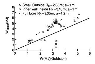
Fig. 70 Diamagnetic energy stored in various 3MA plasmas heated by NBI. The small bore inner wall plasmas give an improvement over Goldston scaling.
