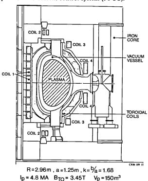
Fig.13: Cross-section of JET showing toroidal and poloidal coils.
