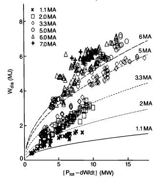
Fig. 71 Diamagnetic stored energy versus input power for ICRH on full bore limiter plasma (H minority). Improvement by up to 50% over Goldston scaling is obtained at 3MA.
