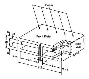
Fig.23: Modified standard JET hypervapotron element.
