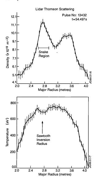
Fig.130: Density and temperature profiles across the mid-plane of JET 19ms after the injection of a pellet.
