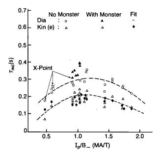
Fig. 73 Incremental confinement time (diamagnetic energy and electron energy content) versus  $I_p/B_r$ . Although the global confinement keeps increasing with  $I_p$  at fixed power input  $\tau_{inc}$  is maximum when  $I_p/B_t \sim I$ .
