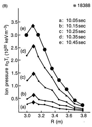
Fig.55 Evolution of (A) ion temperature and (B) ion pressure during a low-density high-temperature inner wall discharge (I=3MA,  $P_{NB}=19MW$ ).
