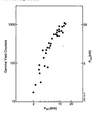
Fig.90: Variation of  $\gamma$ -ray count rate and fusion power from <sup>3</sup>He-d reactions in the energy range (12-20)MeV with applied RF power for a number of discharges. Plasma parameters:  $I_p = (2-4)MA$ ,  $B_T = (3.2-3.4)T$ ,  $\eta = (1.6-4)\%$ . The highest count rate observed corresponds to 60kW of fusion power.
