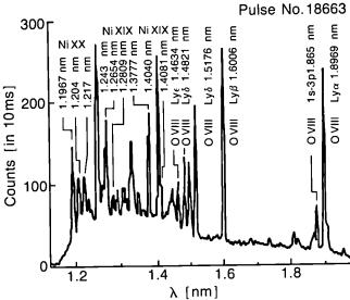
Fig.54 Broad-band spectrum from the double-crystal monochromator, showing Neon-like Ni lines, and H-like and He-like O lines in the range 1.13 to 1.95 nm.
