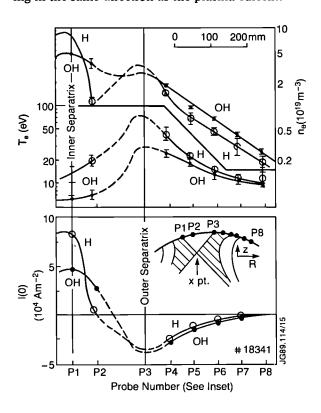
Fig.111: Profiles of density, temperature and ion saturation current in front of the target plates, measured with Langmuir probes mounted in these plates during the ohmic phase of a  $I_p = 4.6\,\mathrm{MA}$  discharge and during an H mode with 14MW of NBI.
