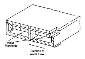
Fig.24: Direct replacment hypervapotron element.
