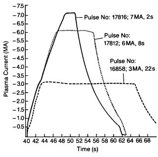
Fig. 61 High current or long flat top discharges. The 7 and 6MA pulses were obtained by ramping simultaneously plasma current  $I_p$  and toroidal field  $B_t$ .
