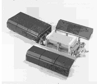
FIG.150: Photograph of one of the JET disruption feedback stabilization poloidal field pick-up coil assemblies. Each assembly contains two 20cm long coils to be mounted vertically in the outer midplane between every two adjacent ICRH antennas.
