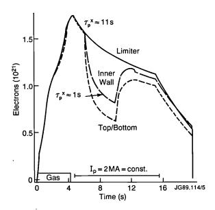
Fig.112: Total electrons in the plasma as a function of time for three discharges, defined by the limiter, the inner wall and the top/bottom of the vacuum vessel.
