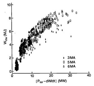
Fig. 66 Stored energy (diamagnetic) obtained with combined heating of full bore plasmas on the belt limiter for 3, 5 and 6MA.
