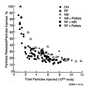
Fig.118: The fractional gas released from the tokamak integrated over a 10 min period after the end of a discharge, as a function of the total number of molecules injected. Results are presented for ohmically heated, ICRH, NBI and pellet injection.
