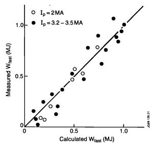
Fig.91: Comparison of measured and predicted total fast ion energy contents of the discharges in the data set. For all discharges, it was assumed that a fraction ( $\mu$ =0.65) of the ICRH power launched by the antenna was coupled to the fast <sup>3</sup>He minority ions.
