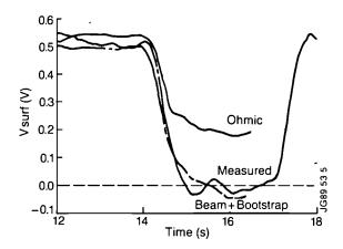
Fig.138: Experimental and theoretical surface voltage traces during a beam heated H-mode. The bootstrap current rises continually during the heating pulse to a level of 0.8 MA. Correspondingly the beam driven current diminishes from 0.1 MA to 0.03 MA due to the density rise.
