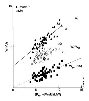
Fig.86: Plasma energy in pedestal and plasma core, respectively, versus total net input power for 3MA H-mode discharges ( $B_T \le 2.7T$ ).
