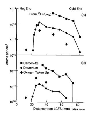
Fig.116: Radial distribution of carbon, deuterium and oxygen deposited on a carbon probe exposed to a single 3 MA discharge (a) constant plasma current exposure (b) current rampdown phase.
