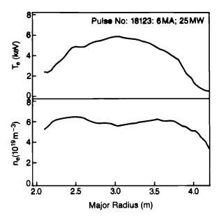
Fig.63 Density and temperature profile during combined heating (25 MW) of a 6.2 MA plasma. Note the flat ne profile and the weakly peaked Te profile.
