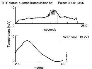
Fig. 40: Diagram of the display provided by the Real Time Processor in the Control Room. The upper curve is the time history of the central electron temperature and the profiles are displayed on the lower left.
