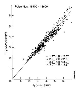
Fig.43: Electron temperature, averaged over the central 0.6m of the plasma, for a large number ( $\sim$  500) of pulses at various magnetic fields. The best fit line has a slope  $T_{LIDAR}/T_{ECE} \approx 0.9$ .
