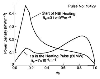
Fig. 68 Heating power density by NBI at 80keV at the beginning of the heating pulse and 1s after.
