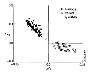
Fig.139: Changes in the second (Y<sub>2</sub>) and third (Y<sub>3</sub>) Shafranov current moments between ohmic and beam heated H-mode phases showing the broadening of the current density profile due to the bootstrap current. For comparison, data are also shown for discharges that have been fuelled by pellets prior to centrally peaked auxiliary heating. In these cases, the current density profile becomes narrower as the heating produces peaked electron temperature profiles.
