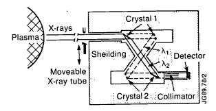
Fig.53 Schematic of the double crystal monochromator.
