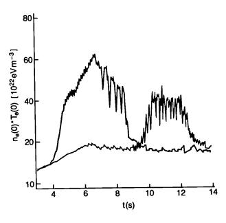
Fig. 76 Product  $[n_e(0)T_e(0)]$  versus time during current rise heating or during flat-top heating. The RF power is 11 MW in both cases. The plasma current starts at 40s and reaches 5 MA at 47s. In the current rise heating case, the RF reached full power at 44.5s; at this time  $I_p$  is 4 MA.
