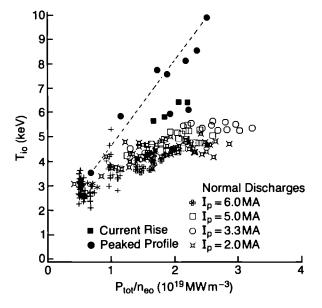
Fig. 74 Central ion temperature during ICRF heating. Best results are obtained with deep pellet fuelling (3 MA) or current rise heating (5 MA).
