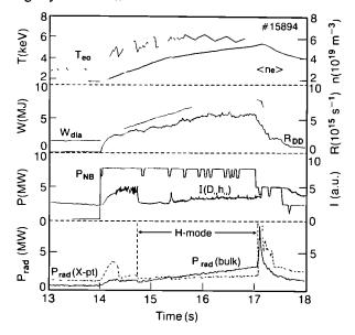
Fig. 79: Time evolution of electron temperature on axis  $T_{eo}$ , volume-averaged plasma density  $< n_e >$ , total plasma energy W, total reaction rate  $R_{DD}$ , neutral beam power  $P_{NB}$ ,  $D_a$  intensity  $I(D_a)$ , bulk radiation  $P_{RAD}$  (bulk) and X-point radiation  $P_{RAD}$  (X-pt) for a 3 MA H-mode discharge ( $B_T$ = 3.1 T).
