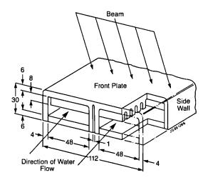
Fig.22: Section through a standard JET hypervapotron element.
