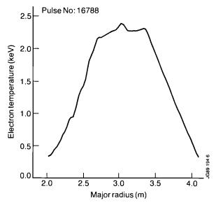
Fig.41: An example of an electron temperature profile measured by the high resolution Michelson interferometer using the first harmonic, ordinary mode. The structure on the profile is within the relative uncertainty of the system calibration (±5%) and so is not thought to be significant.
