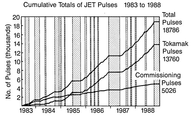
Fig 59: Cumulative total of JET pulses.
