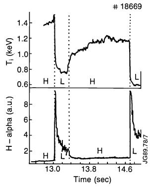
Fig. 56 Ion temperature  $T_i$ , at R = 3.82m and the  $H_{\alpha}$  signal from the plasma edge during a series of H- and L-modes.
