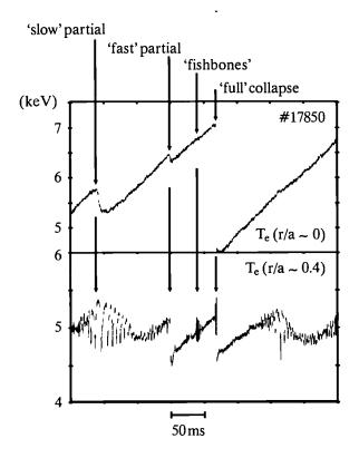
Fig.122: Behaviour of the electron temperature at two radii during a sawtooth cycle in a JET discharge with auxiliary heating. Major commonly observed phenomena are indicated.
