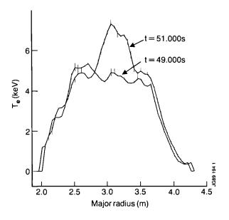
Fig.47: Clearly resolved structure in the LIDAR T<sub>e</sub> profile, evidence of which also appears in soft X-ray and ECE profile data.
