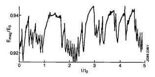
Fig.142: Time behaviour of the normalised magnetic energy,  $E_{mag}/E_o$ , (at a Reynolds number R=6000). Time is measured in units of the Alfvèn time  $t_A(t_o\cong 1000\ t_A)$ .
