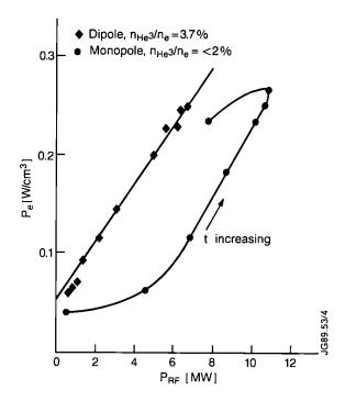
Fig.137: Electron heating power density  $P_{\rm e}$  versus  $P_{\rm RF}$  for minority heating ( $\bullet$ ) and direct heating ( $\bullet$ ). In the former case, the long collisional relaxation time for the minority ions causes both a non-linear response during the RF ramp up and a hysteresis effect as the power is switched off.
