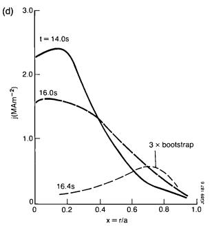
Fig.80: Radial profiles of (a) electron density,  $n_e$ , electron temperature  $T_e$  and ion electron temperature,  $T_i$ , (b)  $Z_{eff}$ , (c) bulk plasma radiation,  $P_{RAD}$  (bulk), and (d) current density during the H-phase of the discharge shown in Fig.79. The dashed line in Fig.80a indicates the radius of the 95% flux surface.
