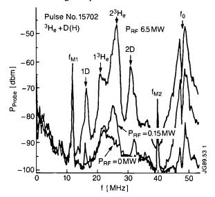
Fig.141: Frequency spectra measured in 3.15 T, 3 MA,  ${}^{3}$ He + D(H) discharges at RF power levels of 0, 0.15 and 6.5 MW. The excitation frequency is 48 MHz and  $f_{M1}$  and  $f_{M2}$  are marker frequencies.
