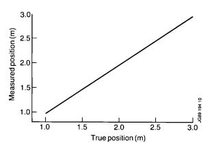
Fig.46: Laboratory test results obtained with one channel (39GHz) of the multichannel reflectometer system. In the tests, the location of a mirror is determined with the reflectometer operating in swept frequency mode and compared with its actual position.
