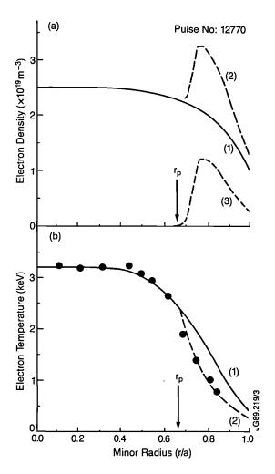
Fig.105: Electron temperature and density profiles immediately before (1) and (2) pellet injection, and the calculated pellet deposition profile (3). The perturbed profiles (2) are those used as the initial conditions for the transport calculation. The circles are the data points from the ECE measurement (KK2).
