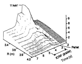
Fig. 64 Electron temperature during the ICRF reheat of deep pellet fuelling. Note the peaked  $T_e(R)$  which suddenly relaxes to a 'monster' at  $\sim 4.5$  s
