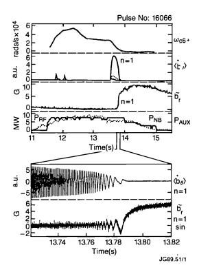
Fig.131: The top trace is the central ion rotation frequency, the second trace is the rectified and smoothed amplitude of MHD oscillations, the third trace is the locked mode amplitude, and in the fourth box are the neutral beam and radio frequency auxiliary heating powers. The expanded time traces show the oscillating MHD activity as the mode locks together with one component of the locked mode amplitude.
