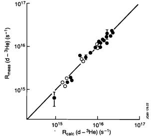
Fig.92: Comparison of measured and calculated  $^3$ He-D fusion reaction rates for the complete data set. Open circles: Plasma current,  $I_p = 2$  MA, filled circles:  $I_p = (3.2-3.5)$  MA. Toroidal field:  $B_T = (3.2-3.4)$  T. The calculated points were obtained with a value of deuterium dilution factor  $(n_d/n_c) = 0.3$ .
