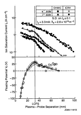
Fig. 106: Radial profiles of saturation ion current  $I_s$  and floating voltage  $V_f$  on the ion and electron drift facing sides of the reciprocating probe in ohmic and ICRF heated discharges.
