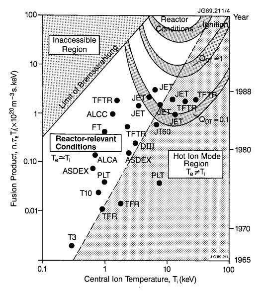
Fig.148: Fusion parameter as a function of central ion temperature for various fusion devices. The mode of operation relevant for a reactor is where the electron and ion temperatures are nearly equal at values between 15 and 50keV. The high density/low temperature region is forbidden due to radiation losses.
