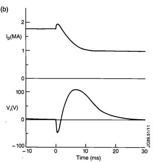
Fig.120: (a) The current increase and negative voltage spike during a 1.8MA disruption and (b) simulation of this process.
