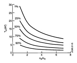
Fig.121: Contours of constant runaway current fraction in the n<sub>e</sub>, T<sub>e</sub> plane for a 1.8MA disruption.
