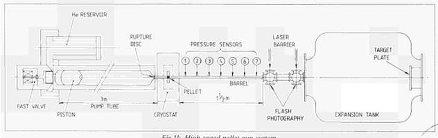
Fig.11: High-speed pellet gun system.
