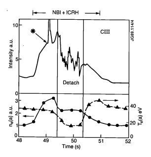
Fig.115: The C III intensity associated with a hot spot on the lower belt limiter and the edge plasma conditions during 28MW combined ICRH and NBI heating.  $I_p = 5$  MA,  $B_T = 3.2$ T, discharge balanced between upper and lower limiters. '\*' denotes hot spot temperature - 1600°C.
