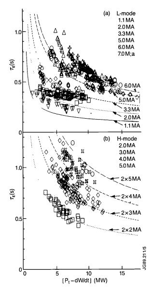
Fig.147(a) L-mode confinement time,  $T_E$ , data versus input power, showing degradation with power. The strong degradation of confinement time and the beneficial effect of plasma current are clearly seen. (b) H-mode confinement time,  $T_E$ , data versus input power showing clear degradation with power. However, confinement is improved by a factor 2 to 3 over the corresponding L-mode case.
