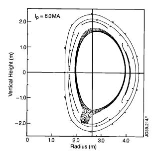
Fig.149: Divertor magnetic configuration at 6MA plasma current.
