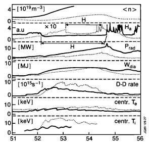
Fig.97: Comparison between an H-mode at medium density (Pulse No:17386, solid line) and one at low density (Pulse No:18757, dashed line). Both discharges have 10MW NBI from t=52s. Note that the  $H_{\alpha}$  signal for the low density case is multiplied by 10.
