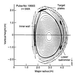
Fig.77: Poloidal flux contours for a 5 MA single-null X-point discharge.
