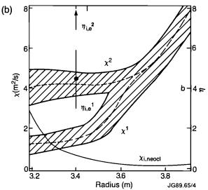
Fig.101: (a) Experimental profiles of  $T_e$ ,  $T_i$  and  $n_e$  for a pellet shot (Pulse No:17279). I refers to the phase of enhanced confinement (t=44.6s), 2 to the following 'normal' phase (t=45s); (b) corresponding 'experimental' thermal conductivity  $\chi$  and values of  $\eta_e$  and  $\eta_i$  at t=3.4m, t=44.6s. The neoclassical (Chang-Hinton) value of  $\chi_i$  at t=44.6s is given for comparison.
