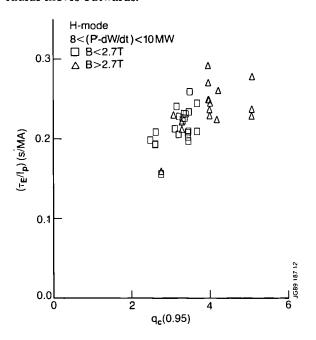
Fig.84: Confinement quality factor  $T_E$  /I versus safety factor at the 95% flux surface  $(8MW \le P_{tot} - (dW/dt) \le 10MW)$ .
