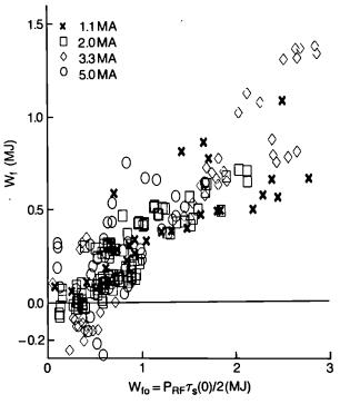
Fig. 72 Perpendicular energy in ICRH generated fast particles versus  $W_{fo} = P_{RF}T_{so}/2$  where  $T_{so}$  is the Spitzer slowing down time in the plasma centre.
