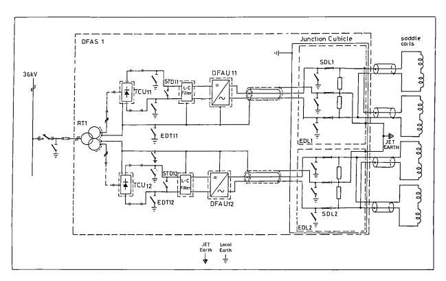
Fig.16: Schematic of the disruption feedback amplifiers.
