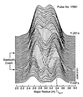
Fig.103: Evolution of the radial profile of soft X-ray emissivity. The background has been subtracted to show the contribution due to injected nickel only.
