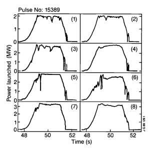
Fig.28: Power launched by each antenna during Pulse No:15389. The total power reaches about 18MW for 2s.
