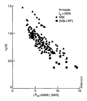
Fig.140: Incremental confinement time  $\tau_{inc}$  for H-mode discharges versus  $P_{tot}$ . The combined (NBI + ICRF) heated plasmas tend to have somewhat lower values of  $\tau_{inc}$  compared with those produced by NBI alone.
