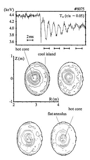
Fig.124: ECE reconstruction of the decay of successor oscillations to a 'fast' partial collapse. The collapse gives rise to an island-like structure which gradually leads to the formation of a shoulder on the temperature profile, apparently by the occurrence reconnection in an annular region about the plasma core.
