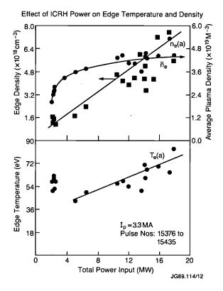
Fig.108: The effect of ICRH power on temperature and density at the last closed flux surface. The change in volume average density  $\bar{n}_e$  is also shown.
