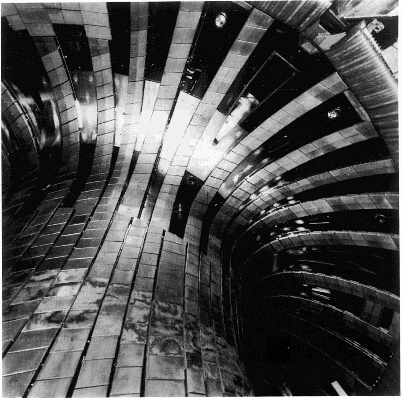
Fig.9 Close up of the vacuum vessel showing the carbon tiles in the X point region.
