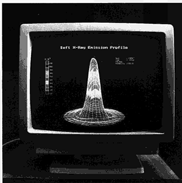
Fig.54: High resolution graphical display of tomographically inverted soft X-ray data generated by the transputer system.
