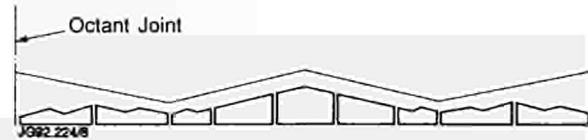
Fig.103: A schematic sectional view through the new beryllium X-point target tiles showing the contouring which shadows tile edges and bolt holes.
