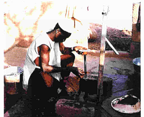
Pump maintenance by an artisan-repairman
