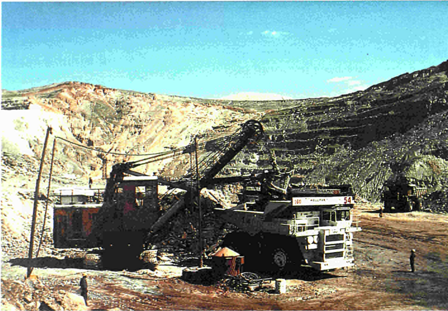
Face shovel loading copper ore, Nchanga open pit
