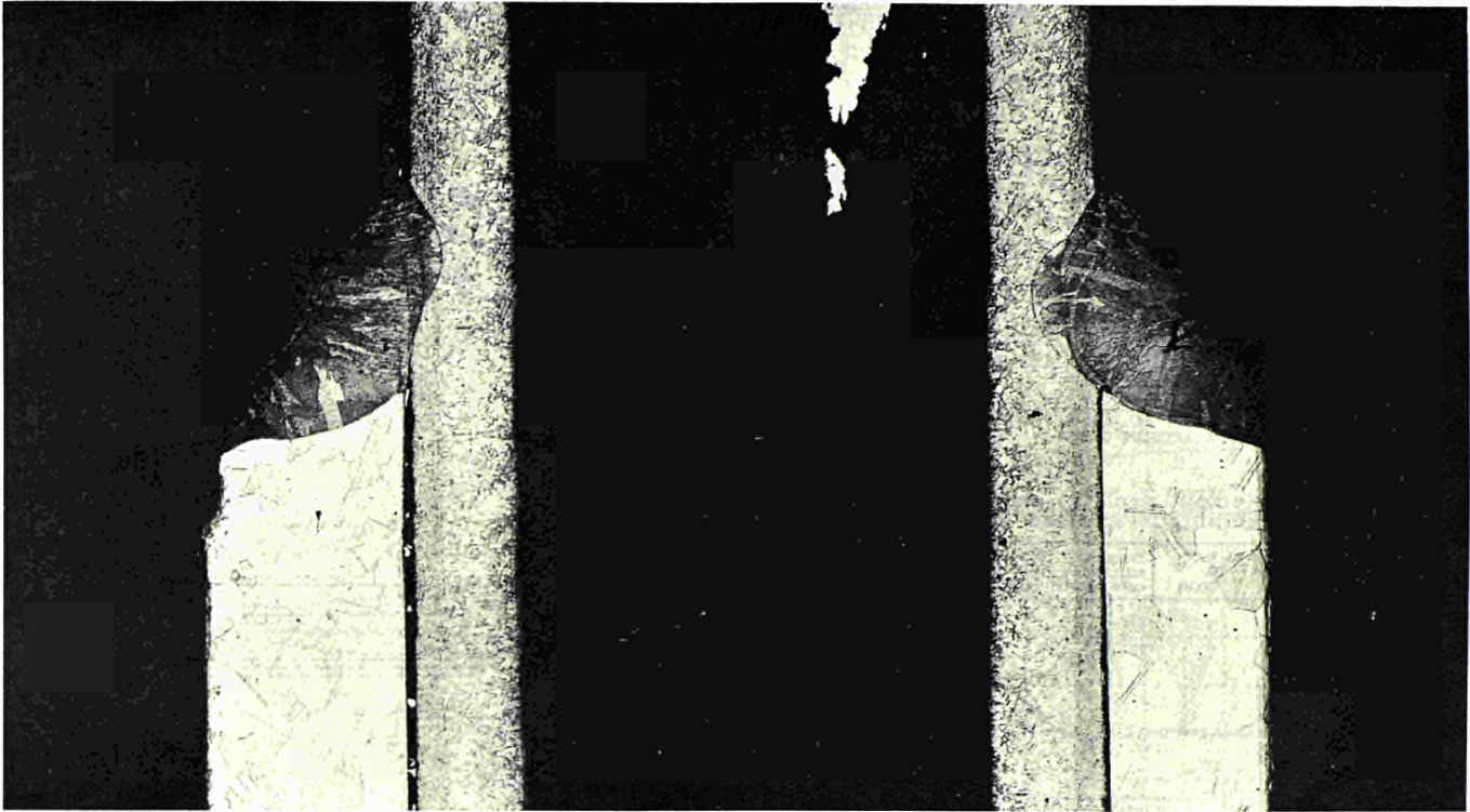
Fig. 2.58 Laser welding. St.st sleeve welded to a st.st-sheathed thermocouple.
