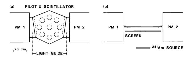
Fig. 12. Schematic view of the scintillator mounting : (a) vertical section, (b) horizontal section
