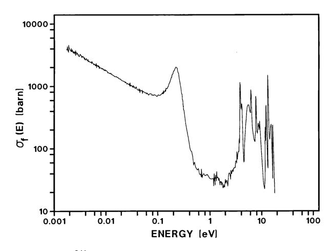
Fig. 7. The  $^{241}$ Pu(n,f) cross section from 2 meV up to 20 eV
