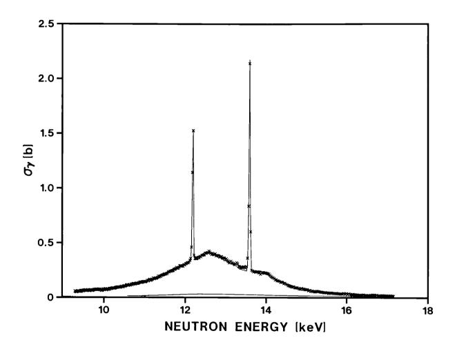
Fig. 8. Shape fit of the triplet of resonances at 12.22, 12.42 and 13.62 keV
