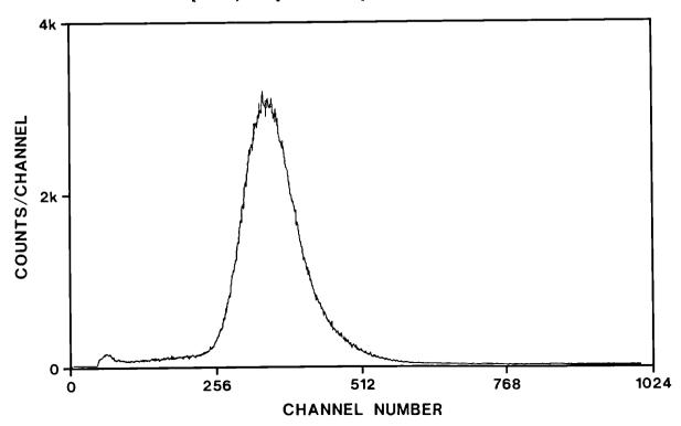
Fig. 10. Pulse height of NE912 in the moderated GELINA beam
