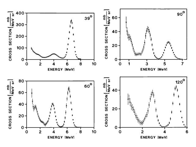
Fig.11. Double-differential neutron-emission cross section of <sup>9</sup>Be for incident neutron energies from 6.5 to 7.1 MeV
