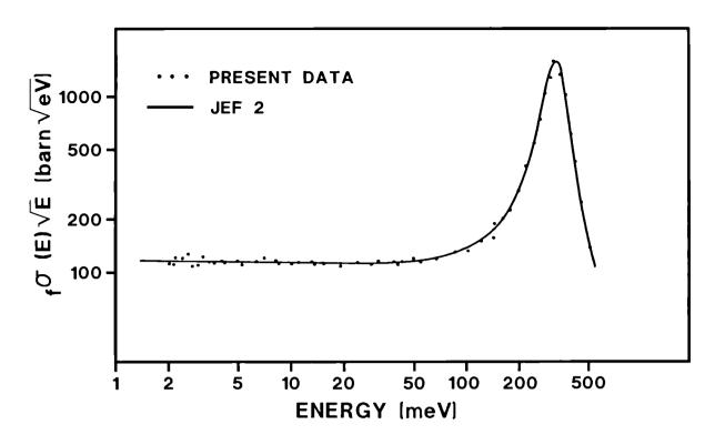
Fig. 6. Comparison of the present <sup>239</sup>Pu(n,f) cross-section data with the JEF-2 data file
