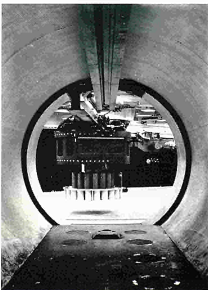
Figure 6: Model of the "loft" handling device; inside of the "loft" seen from a lock-chamber; in the foreground, the loading machine; in the background, right, the breakdown machine.
