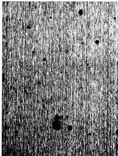
Fig. 1 Pitting corrosion on a sample of 18-8 stainless steel (SERAI, Belgium) Enlarged 12 times
