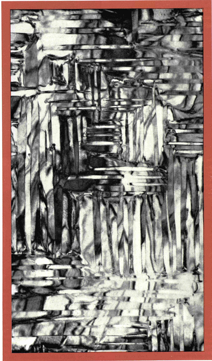
Fig. 6d Nickel oxide nuclei at 920°C (electron microscopy) on copper-nickel sample (1% nickel)
