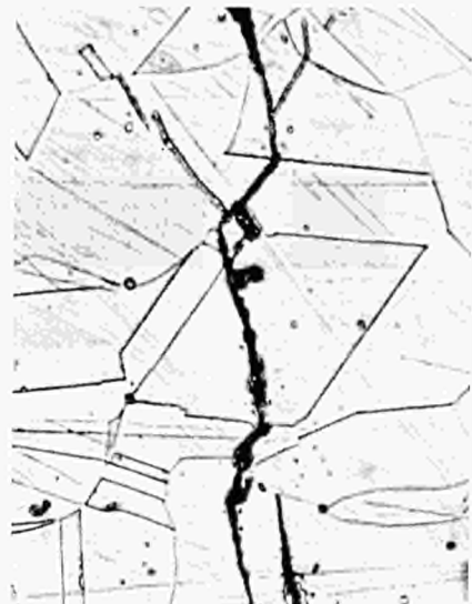
Fig. 2 Crack propagating inwards in an 18-8 stainless steel by transgranular stress corrosion (Metallurgical Chemistry Laboratory, Vitry-sur-Seine, France) Enlarged 800 times
