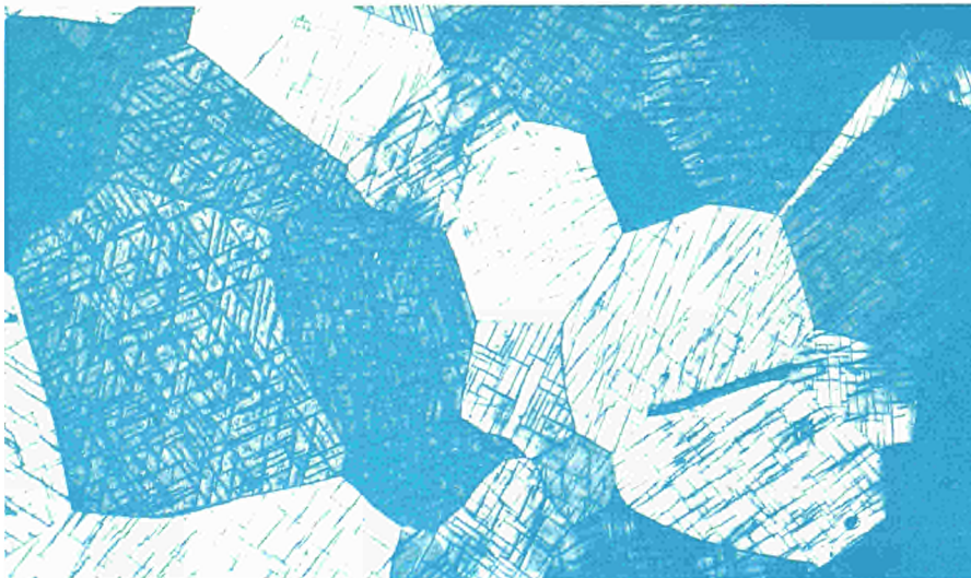
Micrograph of a specimen of stoichiometric natural uranium carbide. Uranium carbide is the reference fuel for the ORGEL concept.
