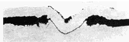
Section of a stainless-steel platelet which has been exposed to steam for 1,000 hours at 500°C. The central part of the photograph represents a zone scored by a diamond point and consequently cold-worked. It will be observed that the oxide layer in this zone is considerably thinner than on the rest of the platelet.
