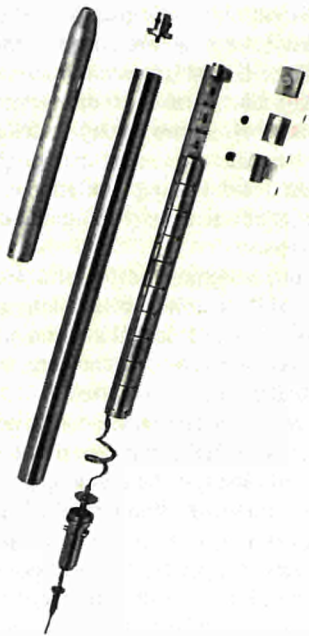
Fig. 6: POM-II irradiation capsule before assembly. In this capsule oxide pellets were irradiated at 100,000 MWd/tonne.
