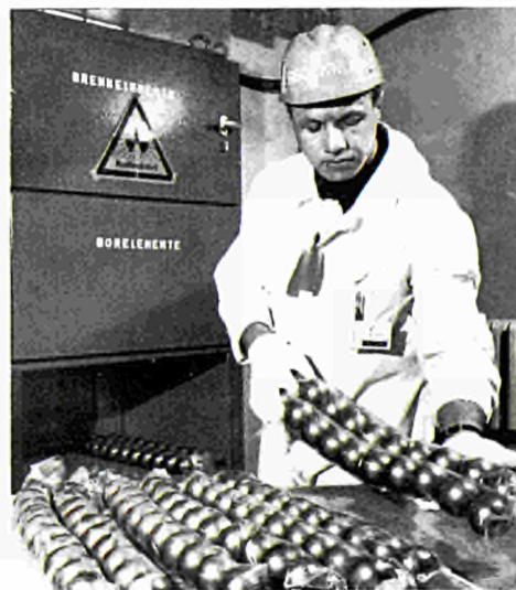
Fuel for the AVR nuclear power reactor. Each sphere contains 1 g of uranium 235 and 5 g of thorium.
