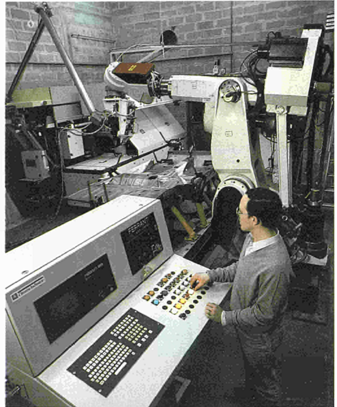
Laser Robot system developed under Brite-Euram project to study the welding of an automotive platform
