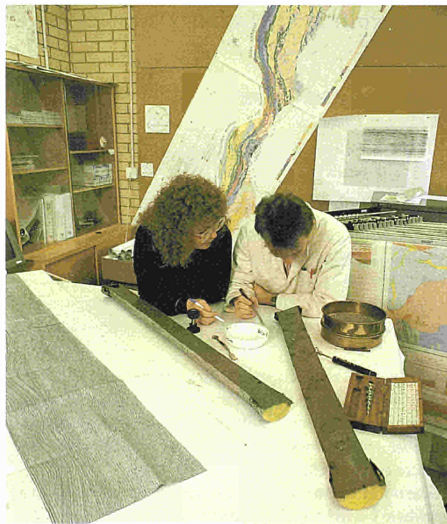
Geologists examining Quaternary borehole cores from the Southern North Sea aided by the use of seismic sections of the area
