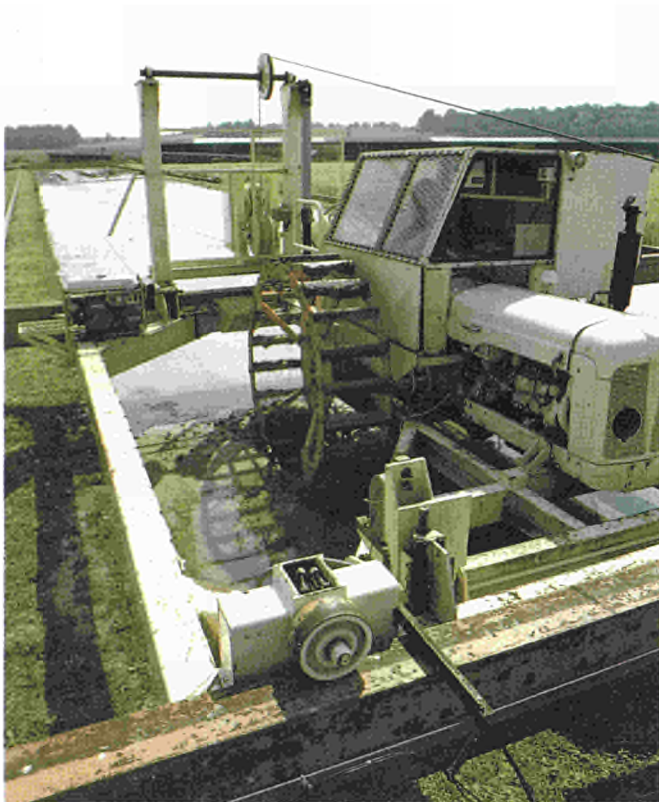
Test facility for investigating the performance of wheels and traction aids in wet paddy fields
