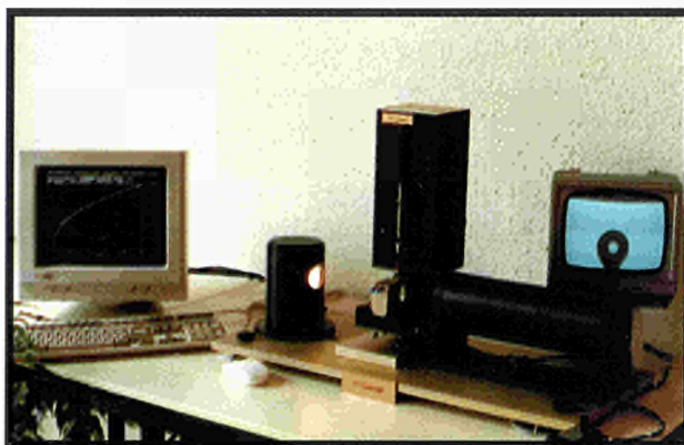
Measuring surface tension between two fluids.
