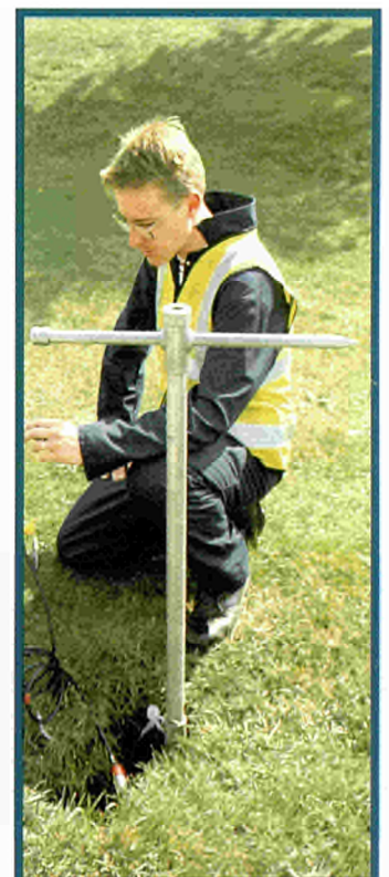
SP257: Close monitoring of predefined leakage control zones can detect leakages and, using instruments, identify their exact location
