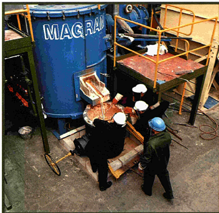
Tapping slag from the MAGRAM furnace.
