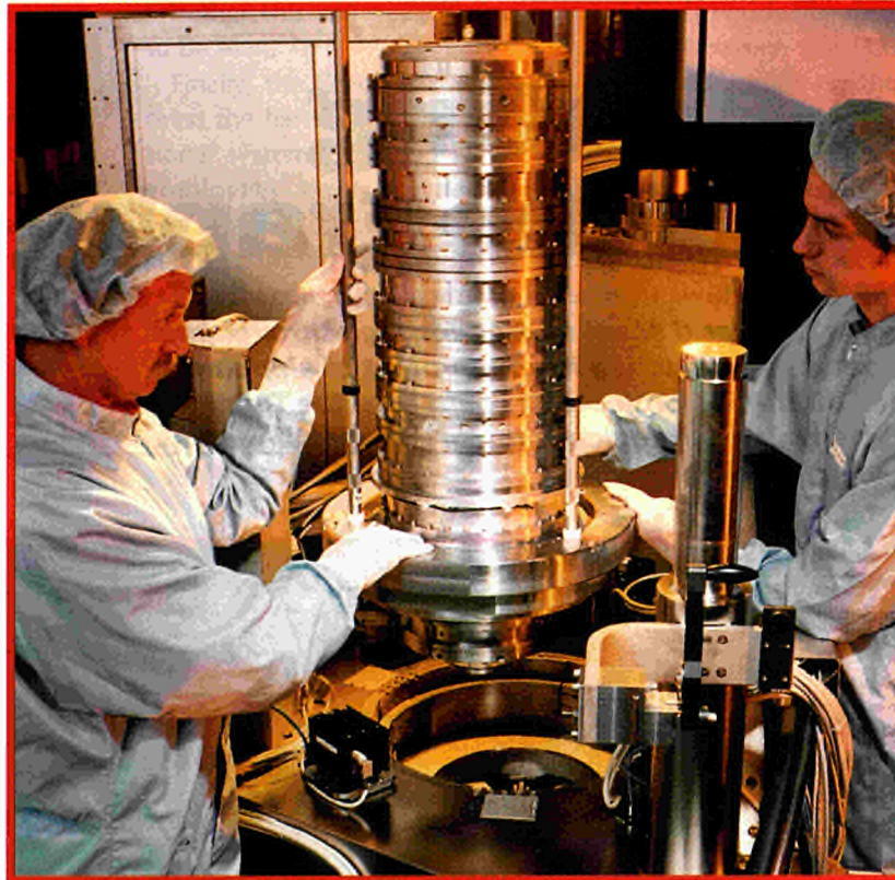
Zeiss DUV projection lens being mounted in an ASML wafer stepper.
