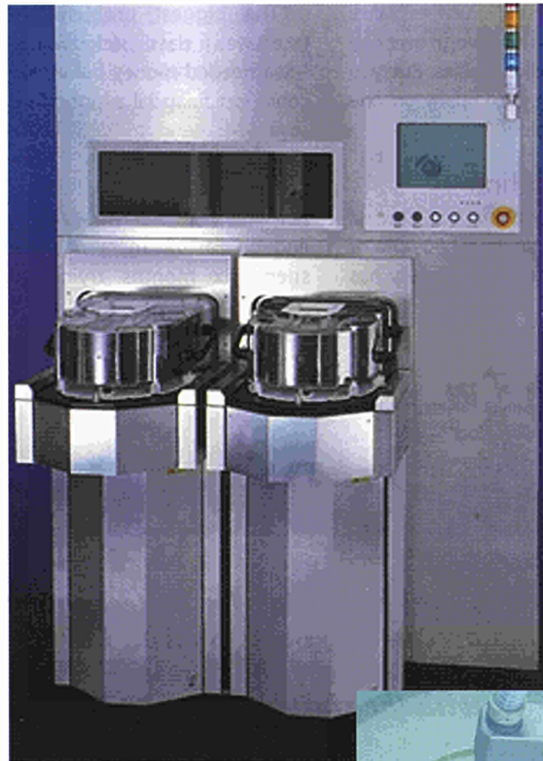
SEZ Semiconductor's Spin Etcher for 300mm wafer processing. Right: inside the process chamber.
