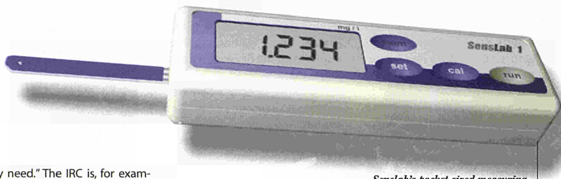
Senslab's pocket-sized measuring device, fitted with one of the company's reusable enzyme sensors for multiple field measurements of glucose, lactate, alcohol or other substances.
