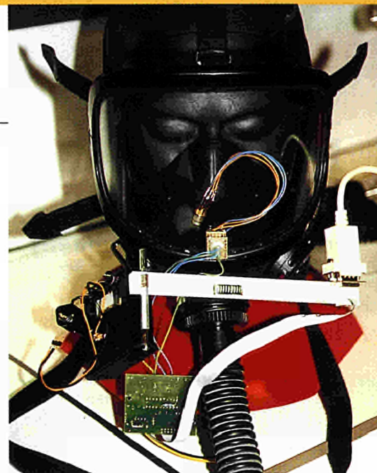
An advanced sensor system, integrated into SNAP's gas masks, will alert the user when a leak occurs or when the filter needs to be changed. Here, a prototype is tested.
