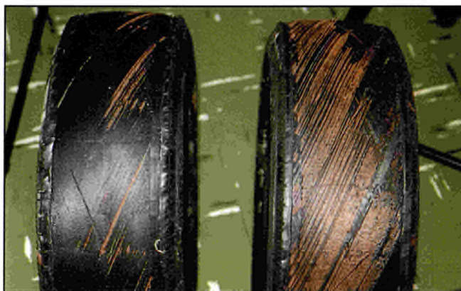
Comparative wear testing: on the right, the very pronounced wear of a traditional tyre with a brass-coated steel structure; on the left, the clearly superior result obtained on a prototype with a zinc/cobalt-coated steel structure.
