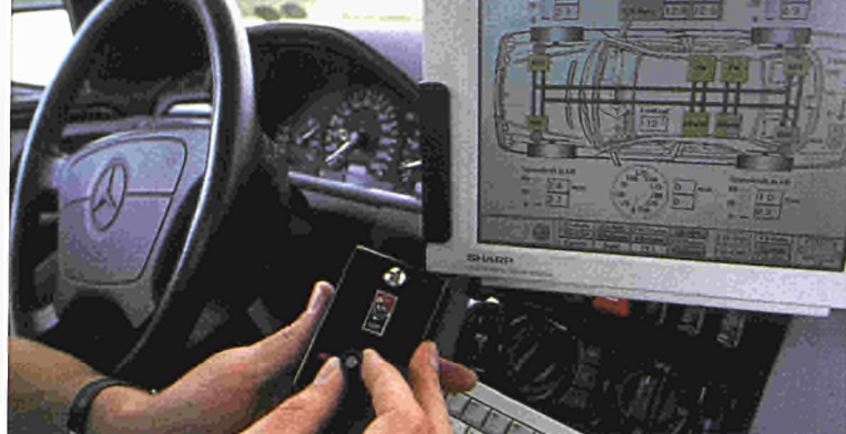
The electric brakes on the test vehicle can be operated by the normal brake pedal or by a manually operated potentiometer for test purposes.
