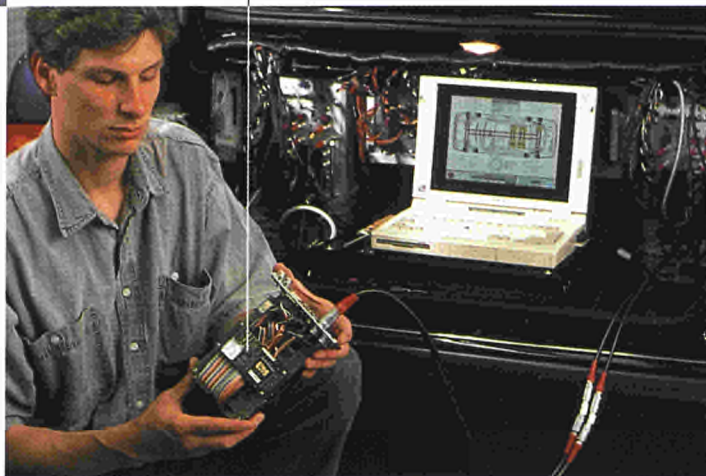
The TTP module on this circuit board is the heart of the electronics innovation. Its functions will be integrated into a computer chip as the development continues.
