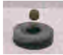
The image shows a classic demonstration of the 'diamagnetic levitation' of a superconducting disc made of an HTS compound when it approaches a magnet. (Photo from the Solid State Physics Group, KTH, Sweden)
