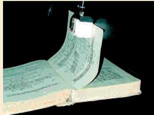
The operating principle of the prototype chemiluminometer which should enable librarians to assess paper degradation.
