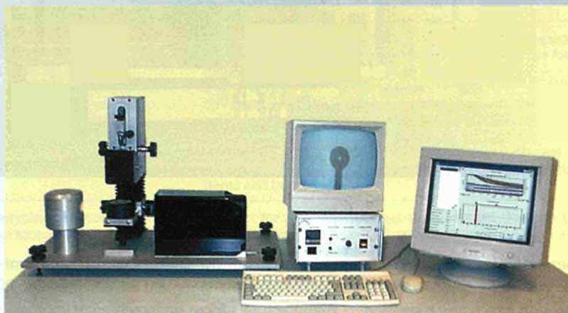
IT Concept's 'Tracker' tensiometer analyses images of a drop of one fluid in a cell containing another, under controlled compression or dilation.
