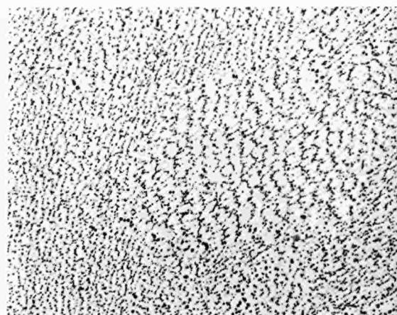
Figure 7: Al-10%Th alloy heat-treated at 600°C for 14 hours, showing globulised ThAl 3 crystals in an α-Al matrix (electropolished; × 240).
