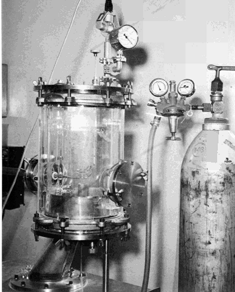
Figure 4: Levitation-melting apparatus for the production of alloys.
