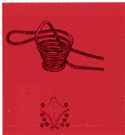
Figure 1: Principle of high-frequency levitation.
