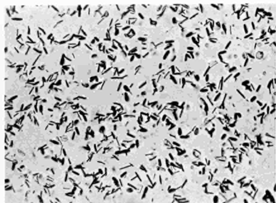
Figure 8: Structure of a cast Al-1%B alloy, showing aluminium-boride needles in an α-Al matrix (electropolished; × 200).
