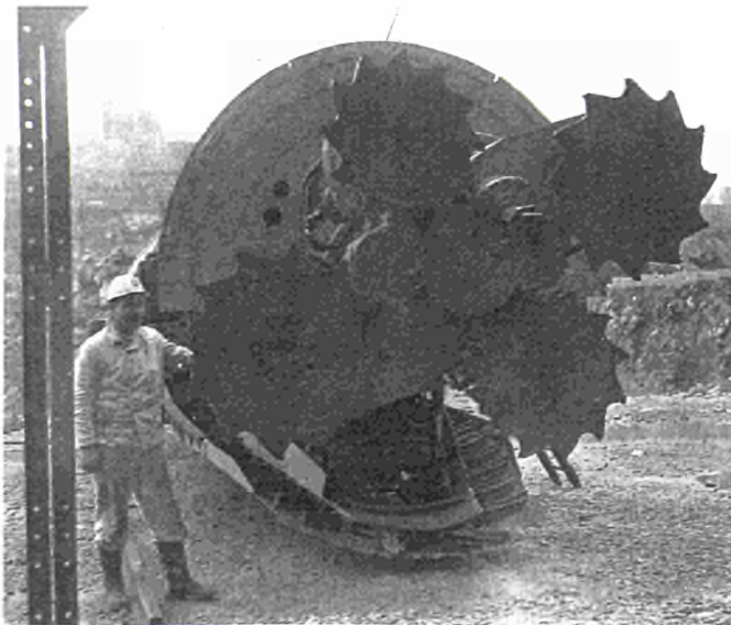
Milling head of Krupp drifting machine for 3.6 m dia roadway.
