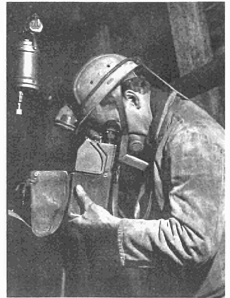
Use of tyndalloscope and konimeter for underground dust-measurement.
