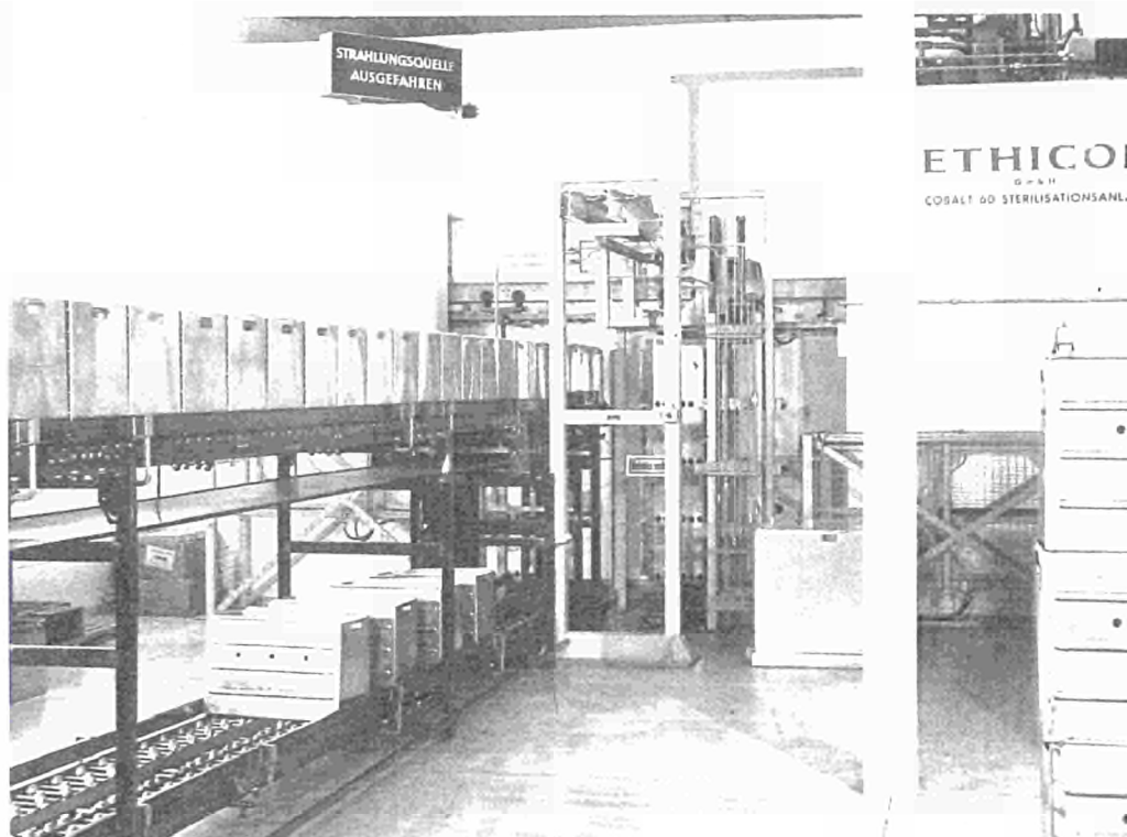
Figure 4: \text{Co}^{60} irradiation device for sterilisation of medical and surgical articles belonging to Ethicon, Hamburg (activity 60,000 Ci).
