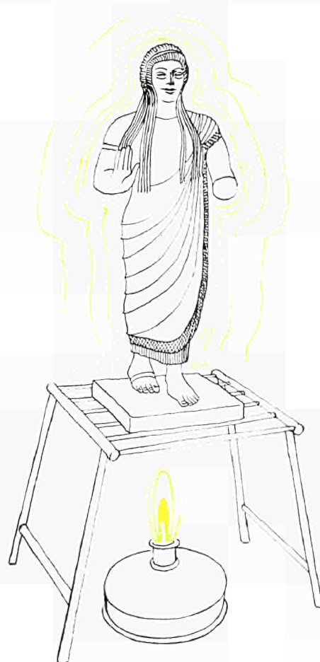
Fig. 5: The thermoluminescence clock in its role of detective. The radiation emitted when the ceramic material was heated showed that this was not an Etruscan statue, but a modern forgery.
