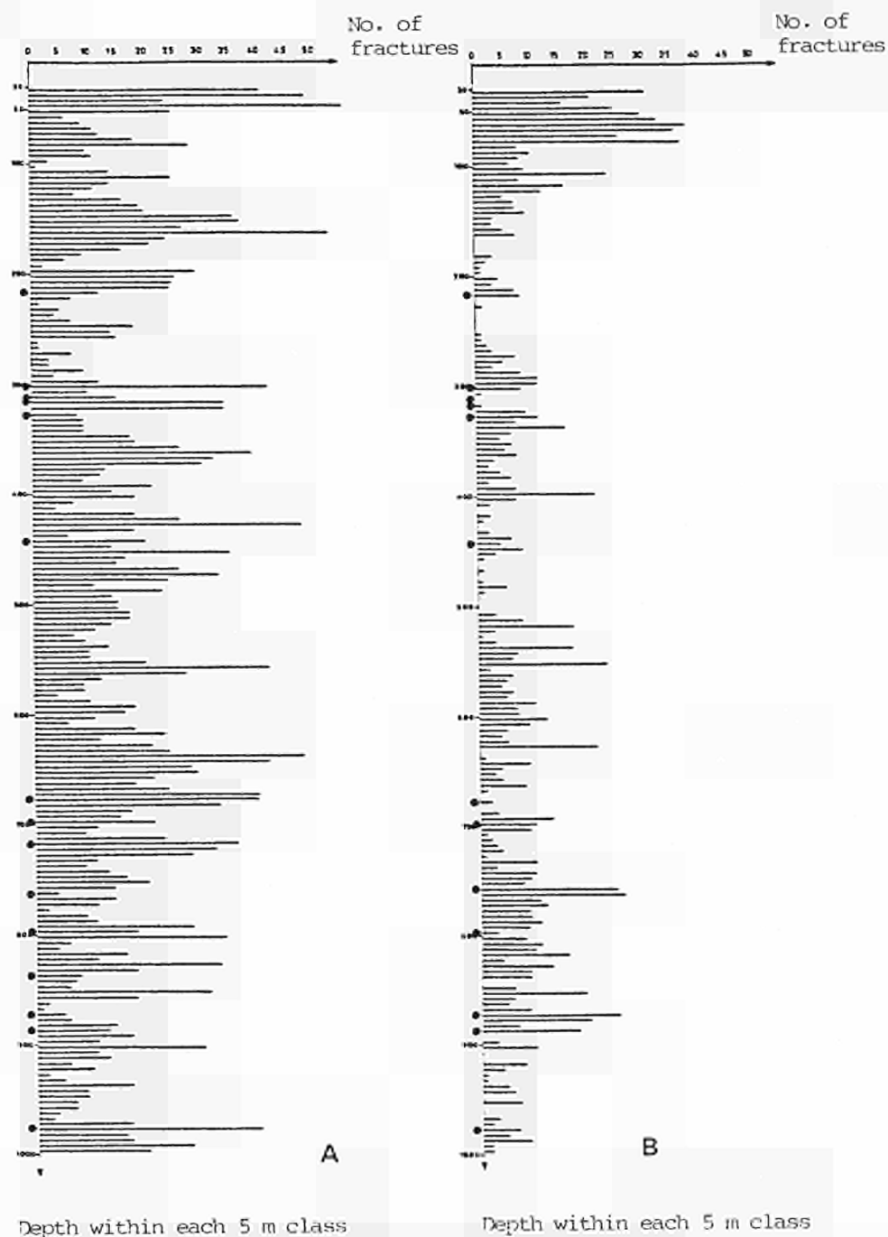
FIGURE 1 - The Auriat borehole : graphs of the number of fractures within each 5 m stretch (after Gros, 1982). A = steeply dipping fractures (dip \geq 60^\circ ) B = gently dipping fractures (dip < 30^\circ ) ● major faults
