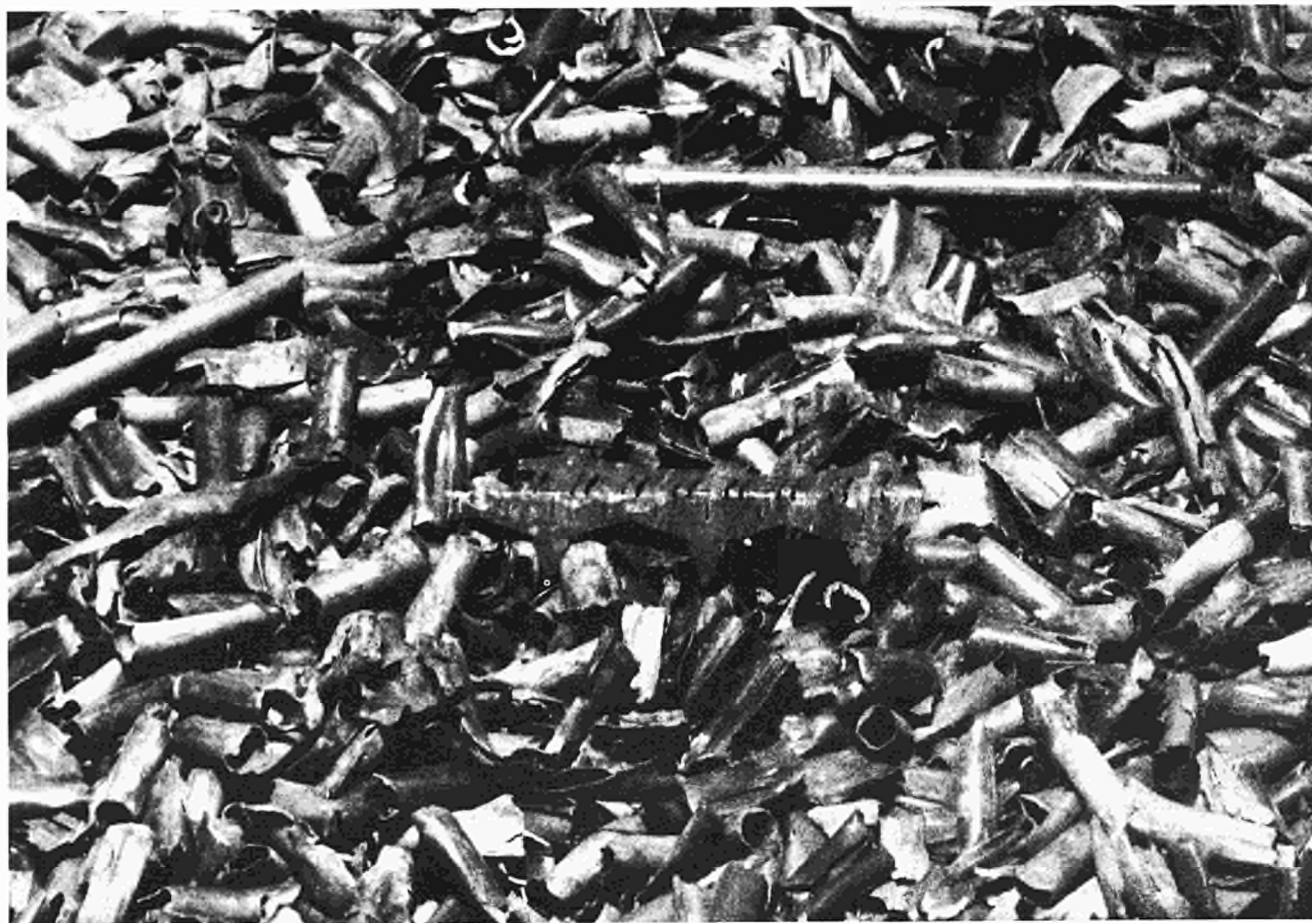
FIG. 1._ GENERAL APPEARANCE OF « OBRIGHEIM » HULLS RECOVERED AT H.A.O. PLANT IN LA HAGUE.
