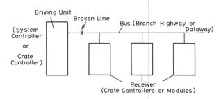
Fig. 3: Sensitivity of bus systems against defective lines.
