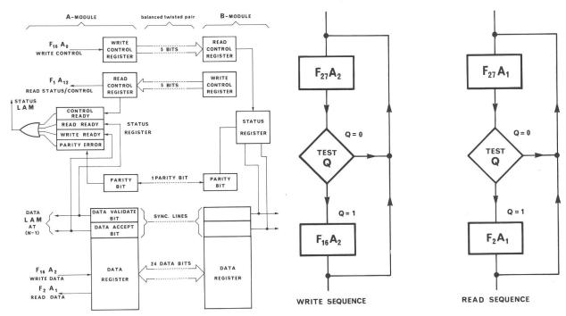
Fig. 3 Block diagram of CAMAC-CAMAC link.
