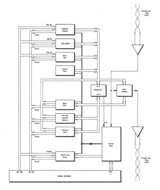
Fig.5 - The Controller, Connects the ring cable to CAMAC
