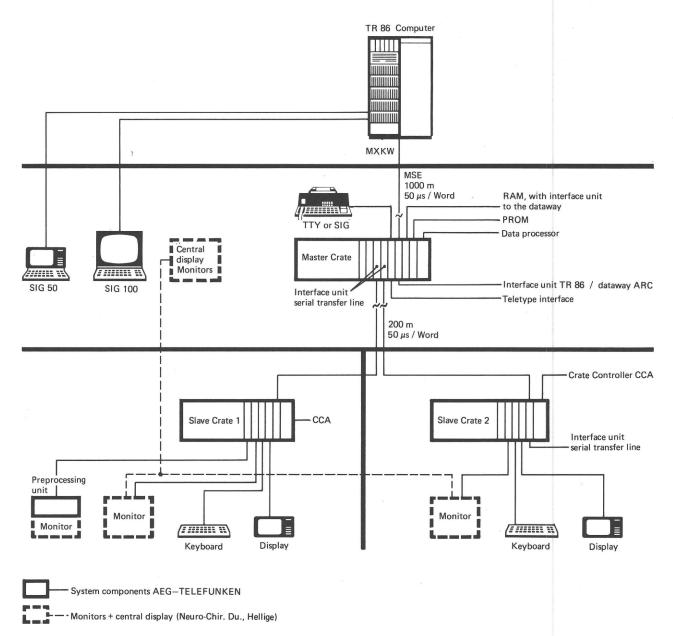
Fig. 4: System Configuration Intensive Care
