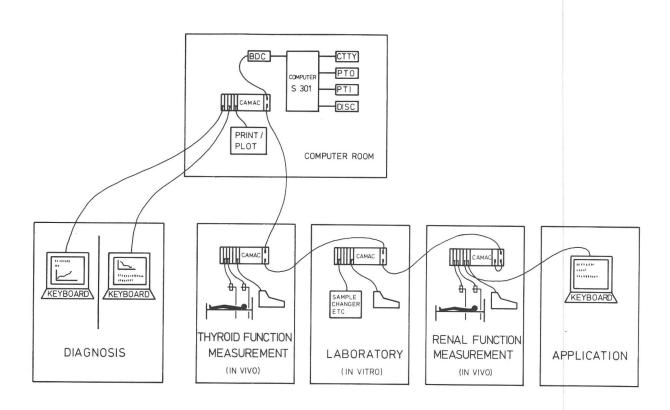
FIG.1: ON-LINE COMPUTING SYSTEM FOR THE DIAGNOSTICS IN NUCLEAR MEDICINE
