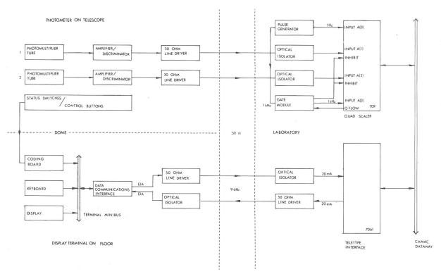
Fig. 5. Photoelectric Photometer Schematic.
