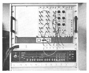
Fig 5 (from the top) CAMAC Crate with CAMAC Modules; patch board for the 7 cables coming from the recorder; Nova computer.
