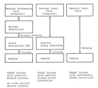
Fig. 1: CAMAC System Structure
