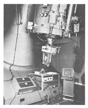
Fig. 2. Photoelectric Photometer Mounted on Telescope.
