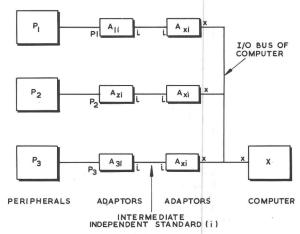
Figure 3. Interfacing through an Intermediate "One-to-One" Standard.
