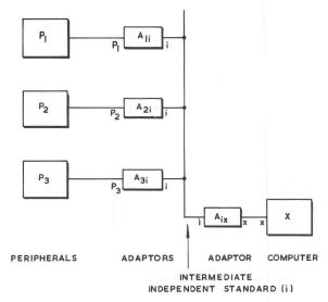
Figure 4. Interface through an Intermediate Many-to-One Standard Highway.
