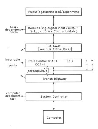
Fig. 1: General structure of the CAMAC system.
