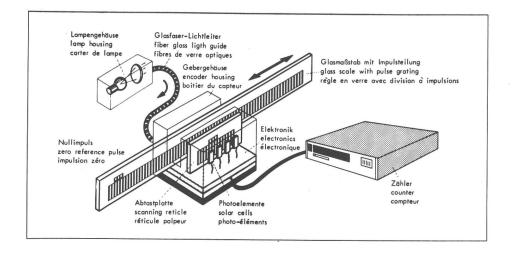
Fig. 4: Principle of a photoelectric incremental position transducer. (Courtesy of Joh. Heidenhain)
