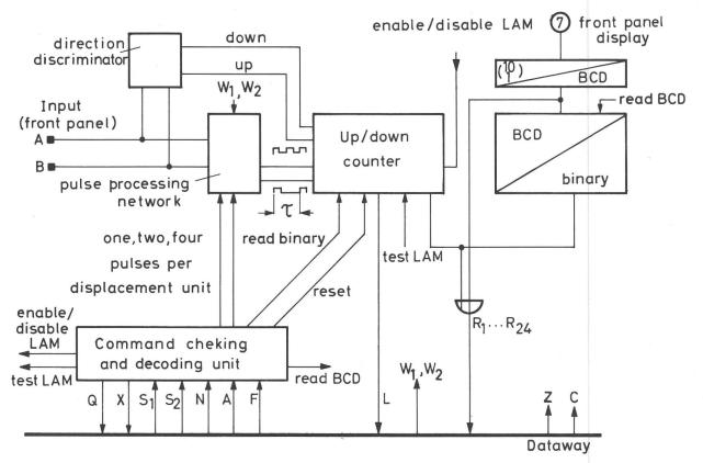
Fig. 6: Block diagram of incremental transducer electronic and display in CAMAC.
