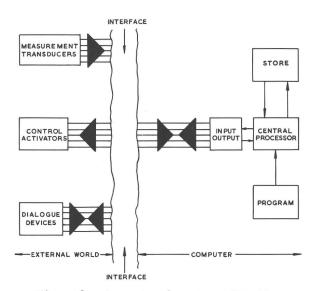
Figure 1. Generalised System Schematic.
