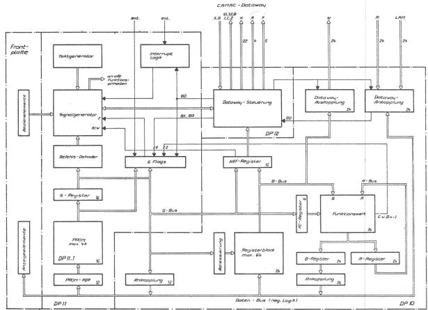
Fig. 2: CAMAC Data Processor Block Diagram
