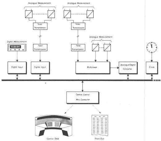
Fig.2 - Data acquisition: Analogue and digital data
