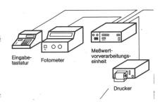
Fig. 3: Pre-processing Unit and Key-board and Printer for Photometers
