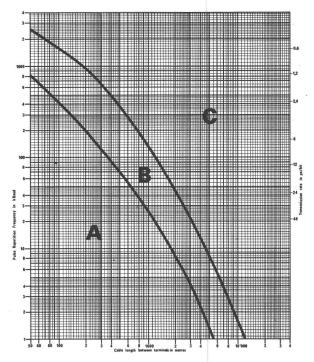
Fig.7 - Transmission rate as a function of distance between terminals
