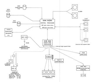
Fig.1 DNPL integrated computer network
