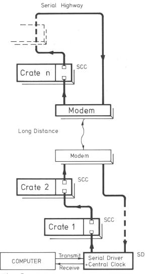
Fig. 7: Serial Highway - Computer System
