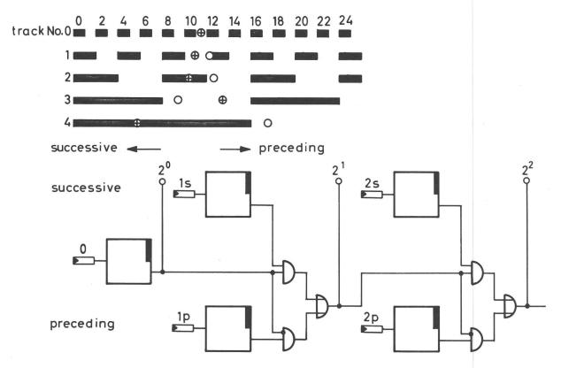
Fig. 7: Binary coded glass scale and V-(Kliever)-Logic
