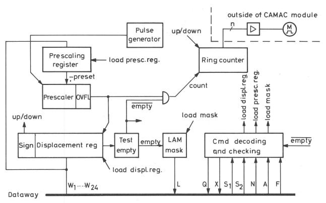
Fig. 9: Block diagram for point-to-point control with stepping motor in CAMAC.
