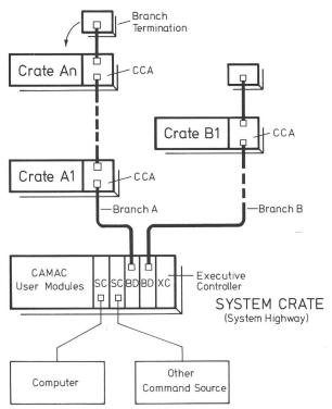
Fig. 6: Concentrated Multibranch / Multisource System with a standard CAMAC crate as System Crate
