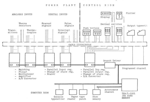
Fig. 1. Block scheme of the Data Logging System.
