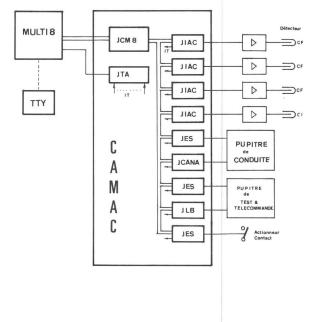
FIGURE II - CONFIGURATION DE L'ENSEMBLE
