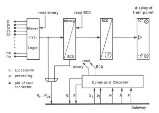
Fig. 8: Kliever-(V)-Logic and display of absolute position transducer in CAMAC.
