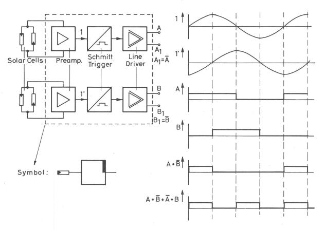
Fig. 5: Transducer electronics and output waveforms.
