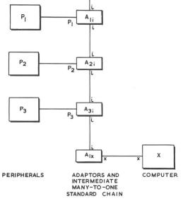
Figure 5. Interfacing through an Intermediate Many-to-One Standard having Chain Connections.
