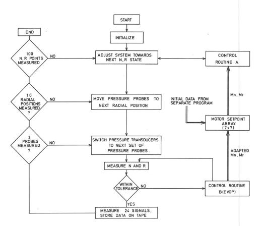
Fig. 3: Control and data acquisition flow diagram
