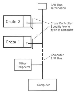
Fig. 3: Dataway - Computer System with dedicated crate controller
