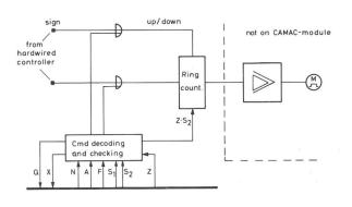
Fig. 10: Block diagram for continuous contour control with stepping motor in CAMAC.
