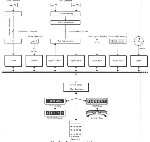
Fig.3 - Data acquisition: Metering data
