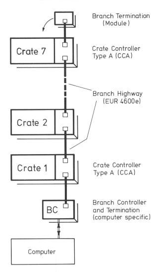
Fig. 4: Branch Highway - Computer System with standard Crate Controller Type A
