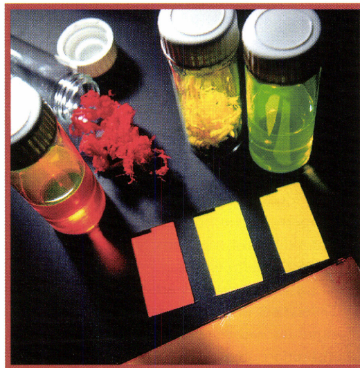
Semi-conducting polymers and their solutions (top), a glass plate with spin-coated polymer thin film (bottom), and three operating displays (centre).
