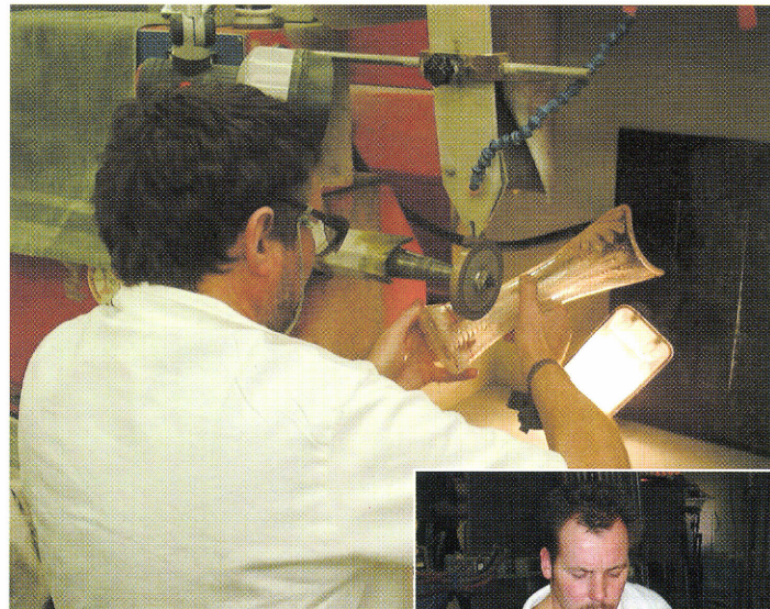
Production of high-value glass-ware at Royal Brierley Crystal. Molten crystal glass (right) produces fumes which condense to form an ultra-fine aerosol. This poses a greater threat to workers' health than the insoluble dust produced during glass cutting (above).
