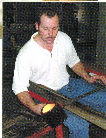
Production of high-value glass-ware at Royal Brierley Crystal. Molten crystal glass (right) produces fumes which condense to form an ultra-fine aerosol. This poses a greater threat to workers' health than the insoluble dust produced during glass cutting (above).
