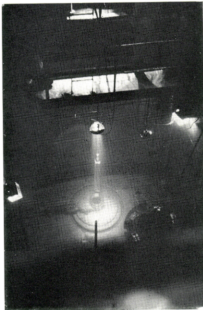
— Introduction of the element containing 12 plutonium-enriched rods into the BR 3 reactor transfer lock.
