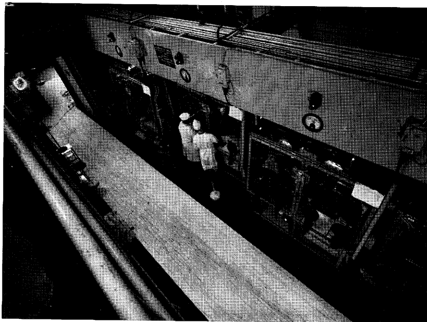
— The glove-boxes of the CEN-Belgo-Nucléaire Group laboratory, in which the plutonium-enriched elements are fabricated.
