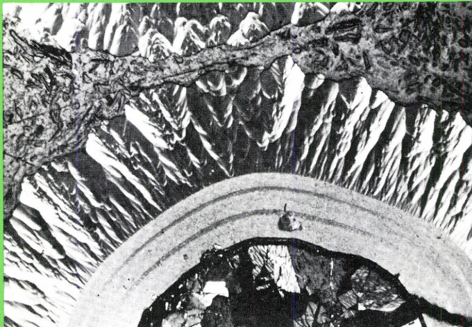
Fig. 4: Basaltic coating deposited at 1,700°C on an initial laminar layer —(ThU) 2 C 2 kernel.
