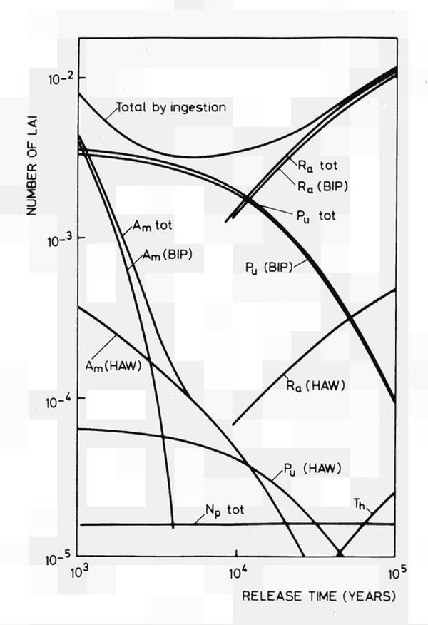
Fig. 4 : NUMBER OF LAI RECEIVED BY INGESTION, AS A FUNCTION OF RELEASE TIME
