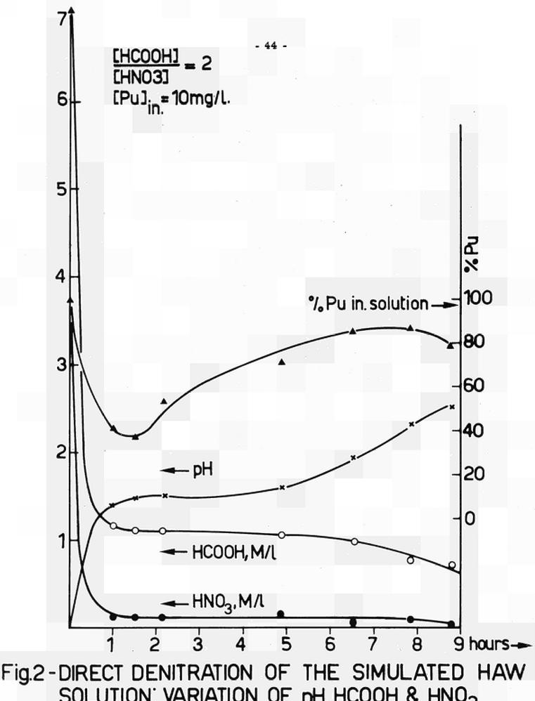
SOLUTION: VARIATION OF pH, HCOOH & HNO3 CONCENTRATION AND OF % Pu FRACTION IN SOLUTION AS A FUNCTION OF REACTION TIME
