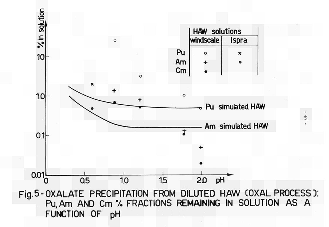
The given quantities (12) correspond to the HAW from 5 t of LWR fuel, burn-up 33,000 MWd/t, decay 150 d. It is assumed that only 10 percent Np is left in HAW
