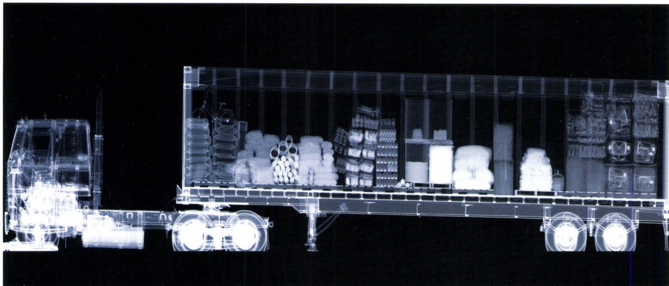
The inside of a truck can be inspected by X-rays.
